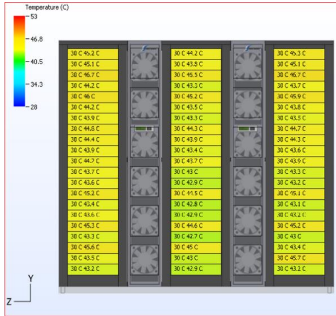
Figure 22 Mean Inlet and Outlet Temperatures for 100% (front) and 50% (rear) Vent Opening Areas of the Two Ducts for Middle Rack.
