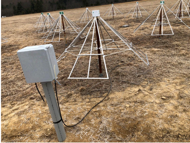
Figure 2.5: An image of an LWA style antenna used in the LoFASM III installation at Green Bank, West Virginia.
