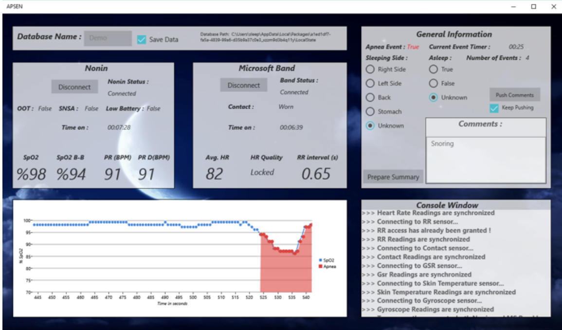
Figure 2.13: APSEN GUI [52]. The user can control the system using this GUI. The GUI provides the ability to connect to the oximeter and the smartwatch (middle two blocks). It also displays the SpO 2 graph in the real time (bottom left block) as well as display the apnea condition. The two blocks on the right provide option to enter user defined annotations if needed.
