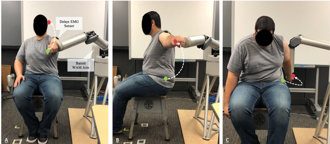
Figure 3.1: Adaptive Robotic Rehabilitation. A user performs three exercises while using the system. The three exercises are Shoulder Flexion (SF) (left), Shoulder Abduction (SA) (middle), and Elbow Extension (EE) (right). The green dot represents the start position. The red dot represents the end position [72]. This system can challenge the user to perform the rehabilitation exercises and help them if and when needed.
