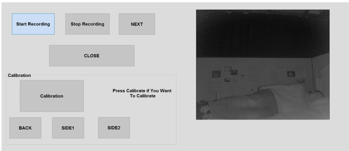
Figure 2.14: Sleeping Position Recording GUI [52]. The user can control the posture detection part of the APSEN system using the controls provided (top left). They can even calibrate the system using the controls at the bottom left. A real-time image is provided on the right to monitor the subject as they sleep.
