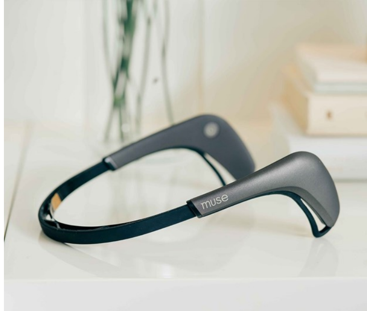
Figure 5.4: MUSE [90] EEG sensor. The user places this sensor on the forehead while playing the cognitive game. This sensor is a nonobtrusive and compact sensor and thus was used to make the system simple and intuitive. The EEG data is extracted from the sensor, which is then used to study cognitive fatigue.
