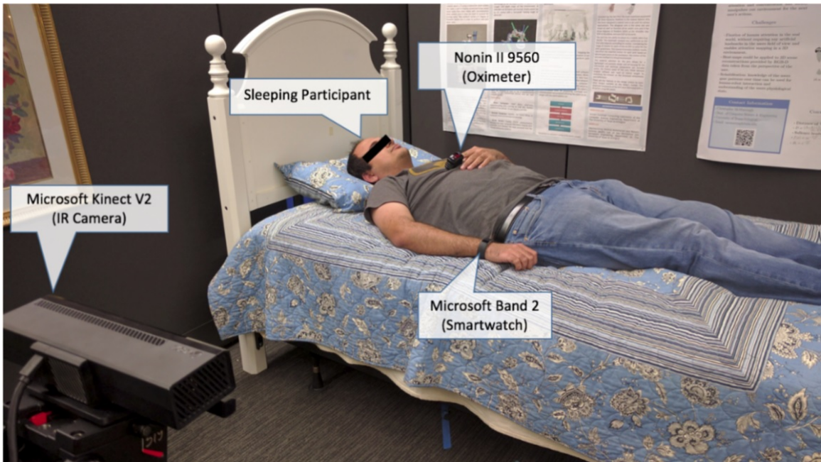
Figure 2.10: APSEN System Setup [52]. The user wears the oximeter and smartwatch and sleeps in front of the IR camera.
