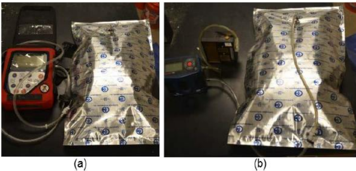
Figure 3. 16 (a) Determination of gas composition by Landtec GEM 2000, (b) Gas volume determination with SKC grab air sampler and Defender 510.
