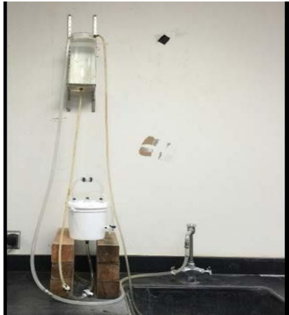
Figure 3. 10 Leak test of reactors
