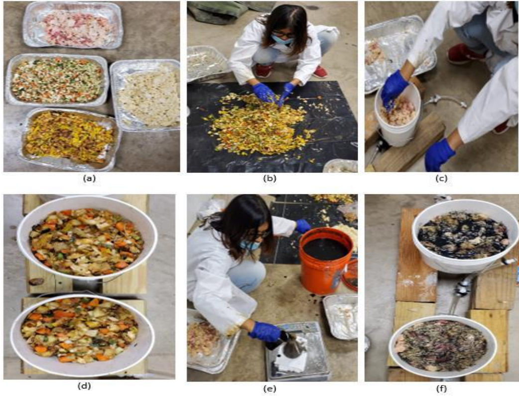
Figure 3. 11 (a) Four types of food waste, (b) Mixing waste; (c), (d) filling reactors (e) weighing sludge and (f) mixing sludge
