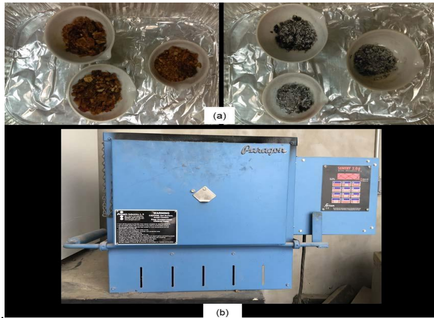
Figure 3. 13 Volatile solids determination (a) samples before & after burning, (b) muffle furnace
