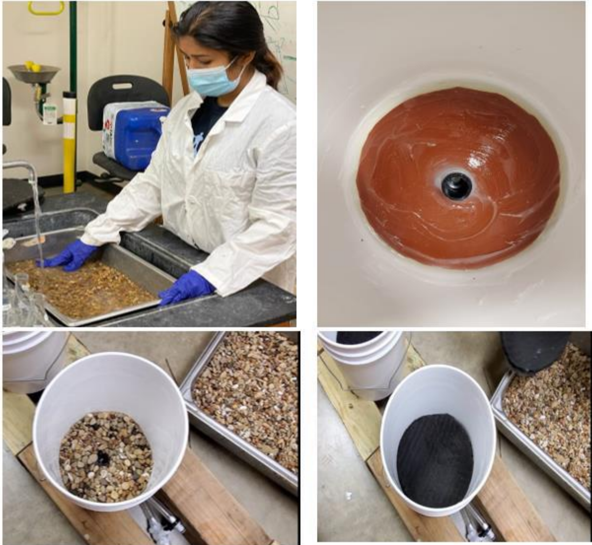
Figure 3. 9 Pea gravel and geo-composite inside the reactor bucket
