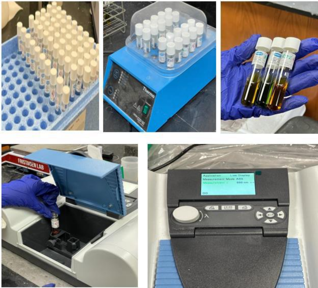
Figure 3. 18 Chemical oxygen demand (COD) determination: (from top left) COD vials, heating in the digester, vials after heating; (from bottom left) putting vials in the spectrophotometer, absorbance measurement by spectrophotometer.
