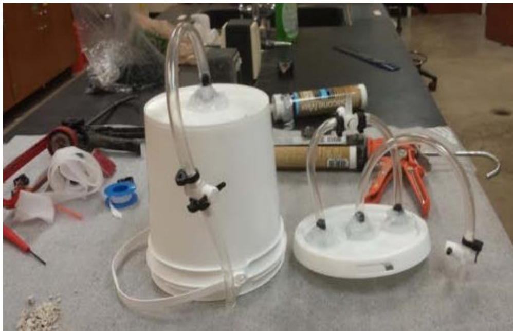
Figure 3. 8 Tubing and valves connected using clamps and silicon sealant.
