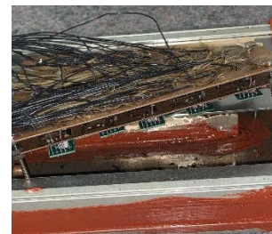
Testing board inserted to the oil-bath
