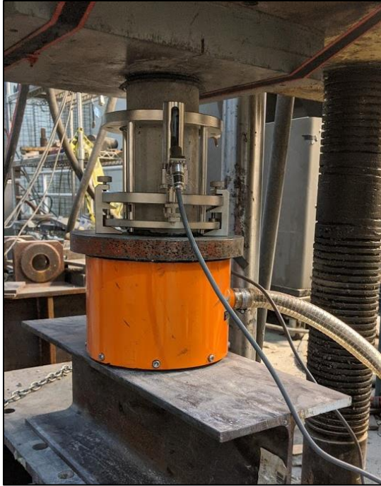
Fig 5.1: Concrete compressive testing of the cylinders
