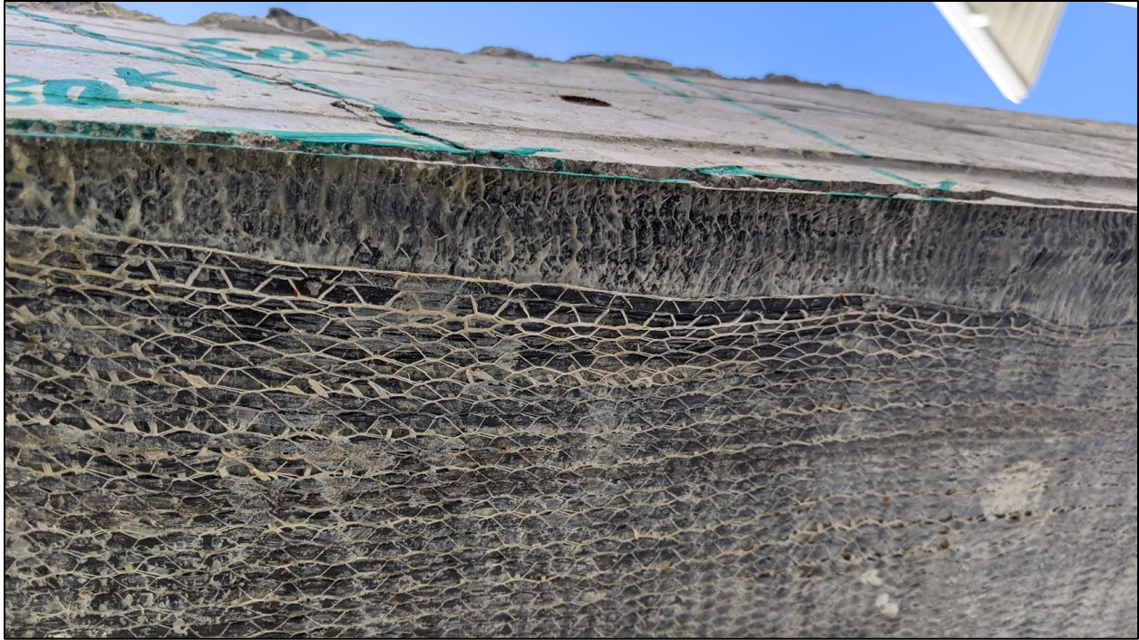
Fig 5.6: Stretching of unidirectional fiber in transverse direction
