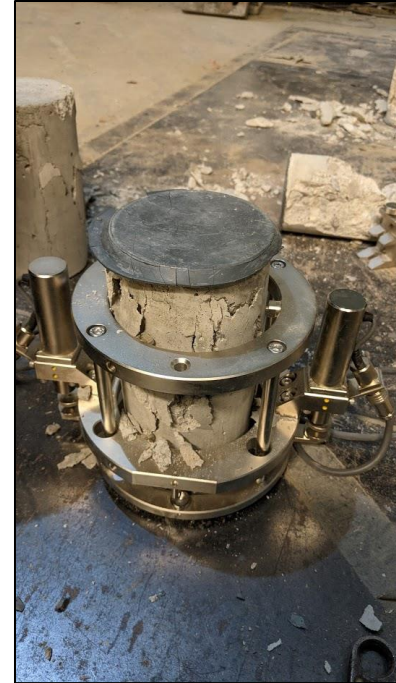
Fig 5.1: Concrete compressive testing of the cylinders
