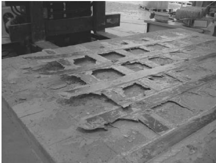
Fig 2.7: Debonding failure of CFRP strengthened slab (Limam et al., 2003)
