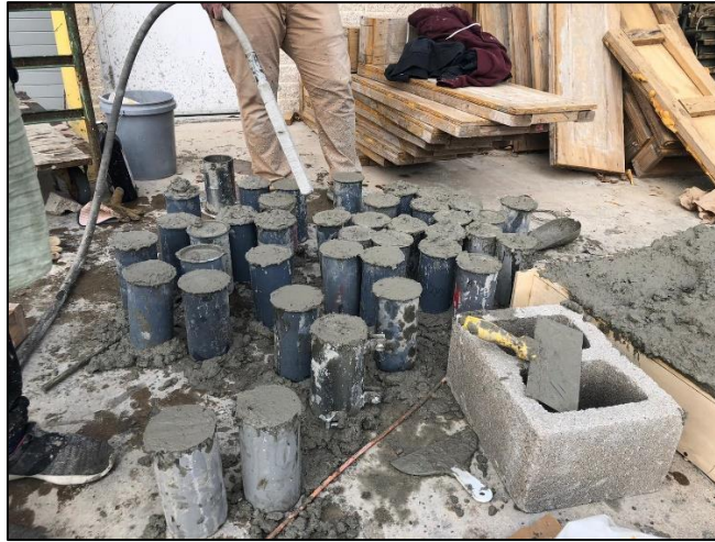
Fig 3.4: Pouring of concrete cylinders
