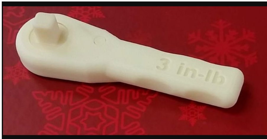
Figure 5: A ratchet wrench fabricated onboard the ISS using AM [55].
