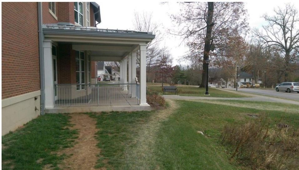
Figure 10 - Obstruction used to deter use of Desire Path, Encourages separate Desire Path
