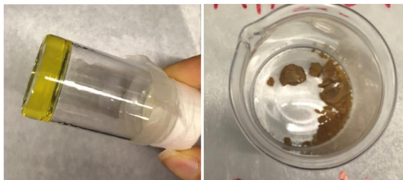
Figure 1. PMHS-DVT yellow wet gel obtained after 3 days, shown as a band at the bottom of the inverted vial (left) and the dark brown, fragile polymeric aerogel particles obtained after supercritical removal of CO 2 (right).
