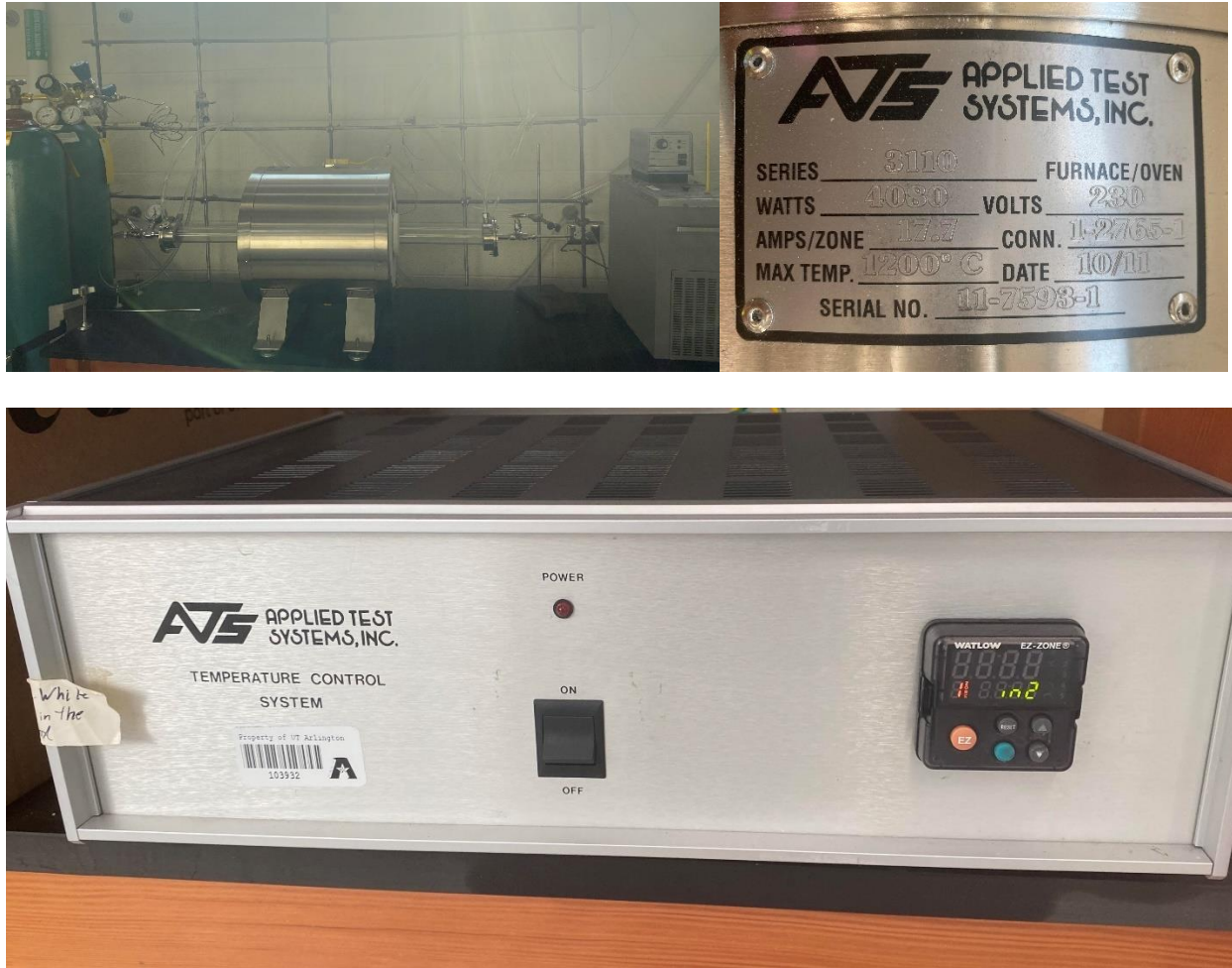
Figure 2-5. The tubular furnace (top) and its temperature control system (bottom).
