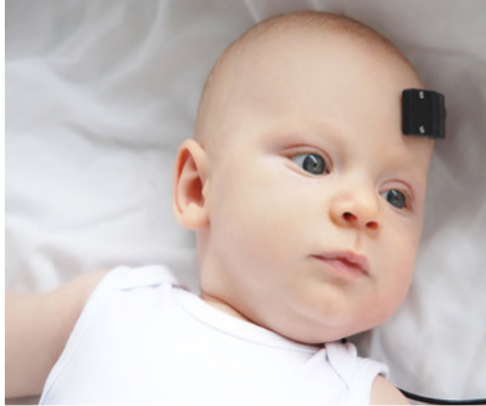
Figure 2.1. A type of fNIRS machine, shows the appropriateness for infant study (Artinis medical SYSTEMS: Fnirs and NIRS devices-portalite mini, n.d.).
