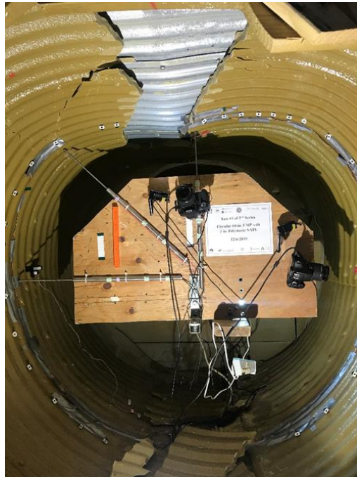
Figure 3-68 Crack in 1 in. thick liner after the completion of test for 1 in. thick liner (Source: CUIRE Laboratory)
