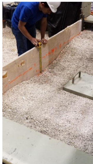
Figure 3-48(Left) Movement of the CMP monitored during the invert removal through Digital Image Processing (Darabnough Tehrani, et al., 2020), (Right) Settlement of soil after invert removal
