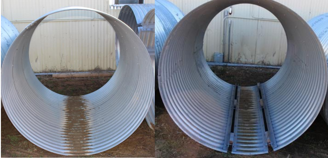
Figure 3-25 (a) Intact CMP (b) CMP with invert removal arrangement
