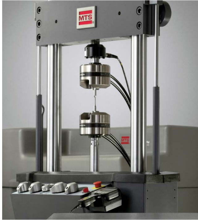
Figure 9. 100 KN MTS Landmark servo-hydraulic test platform.
