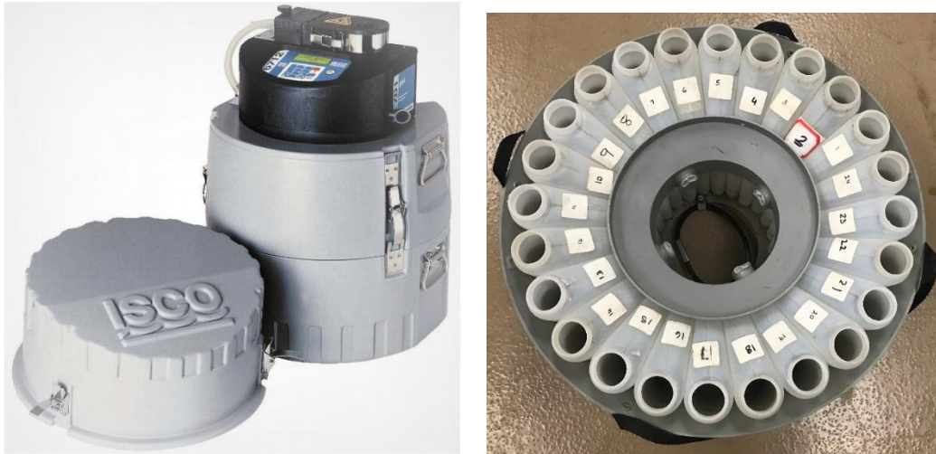
Figure 3-6: (a) ISCO,(b) Sampling bottles
