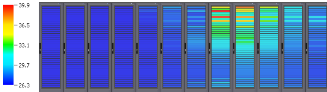
Figure – 22: Server inlet air temperature distribution inside cold aisle
