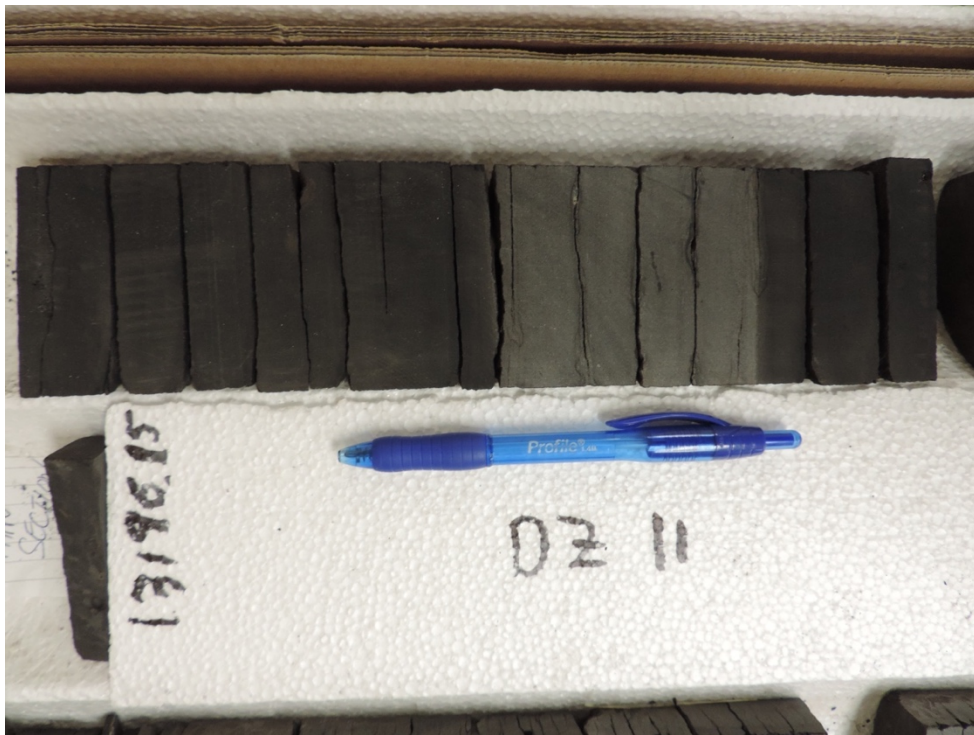
Figure 6: Volcanogenic ash beds (lighter in color) and calcite in kerogen in the subsurface Eagle Ford core Well 8.
