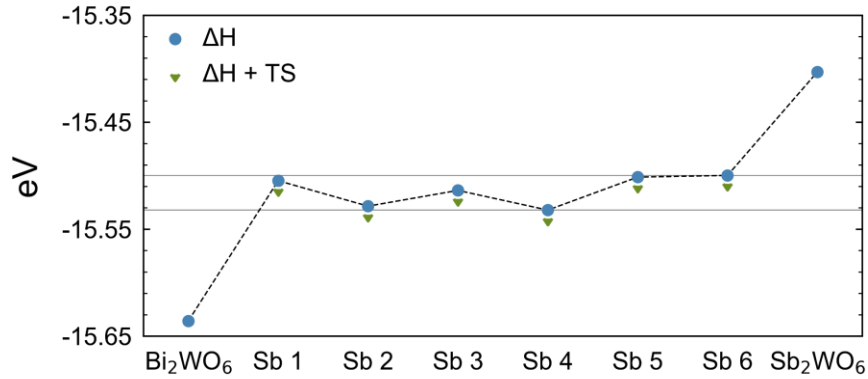
Figure 4.4. Calculated formation enthalpies. Configurational entropy (TS) is added for \text{BiSbWO}_6 via eq. 2. Formation enthalpies for \text{BiSbWO}_6 lie within a narrow \sim 30 meV band marked by solid lines.
