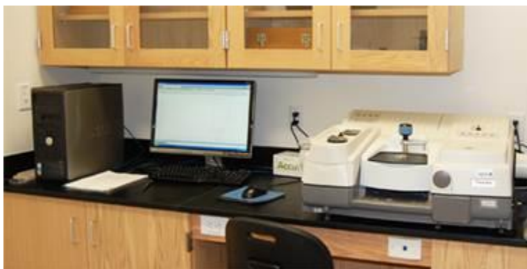
Fig. 4.9: Thermo Nicolet 6700 FTIR Spectrometer [79]
