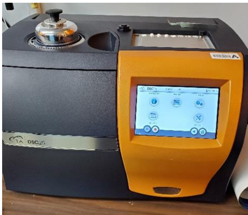
Fig. 4.8: Differential Scanning Calorimetry Setup.
