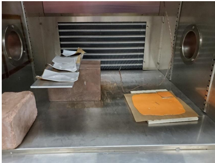
Fig. 4.17: TIM samples inside the thermal chamber.
