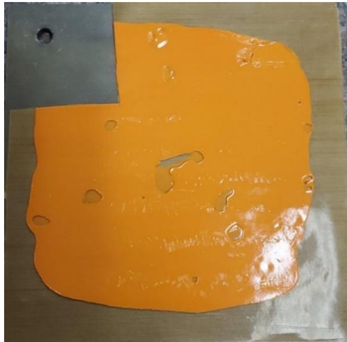
Fig. 4.16: Cured silicone free TIM sample
