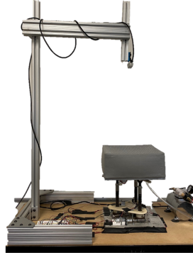
Figure 3.3: Experimental setup of data collection from prototype force bed unit.
