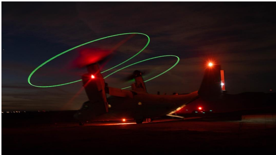
Figure 3-9 Visual representation of the rotor tip path planes for a V-22 Osprey.
