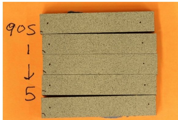
Figure 6. SBS specimens of an unstitched NCF composite.
