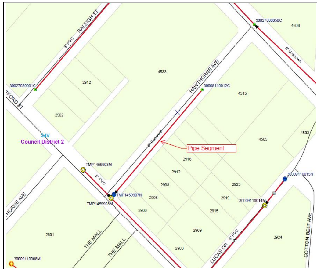
Figure 4-16 Sanitary Sewer Pipe Segments
