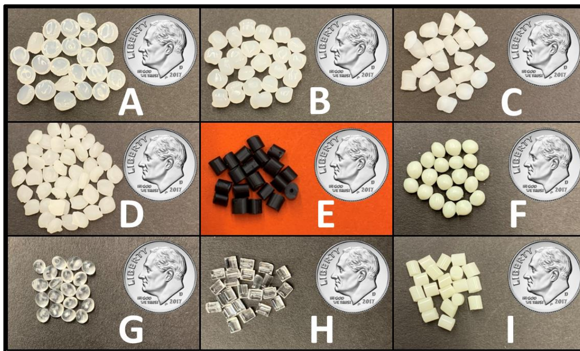
Figure 148. Virgin Plastic Pellets: Pre-CryoMilling 20 pellets shown with a dime for size comparison: Comparing example photos of nine different types of plastic; [A] LDPE; [B] HDPE; [C] PPRp; [D] TPUr ; [E] HIPS ; [F] PETE; [G] PETG; [H] PCRb; and [I] ABSt particles.
