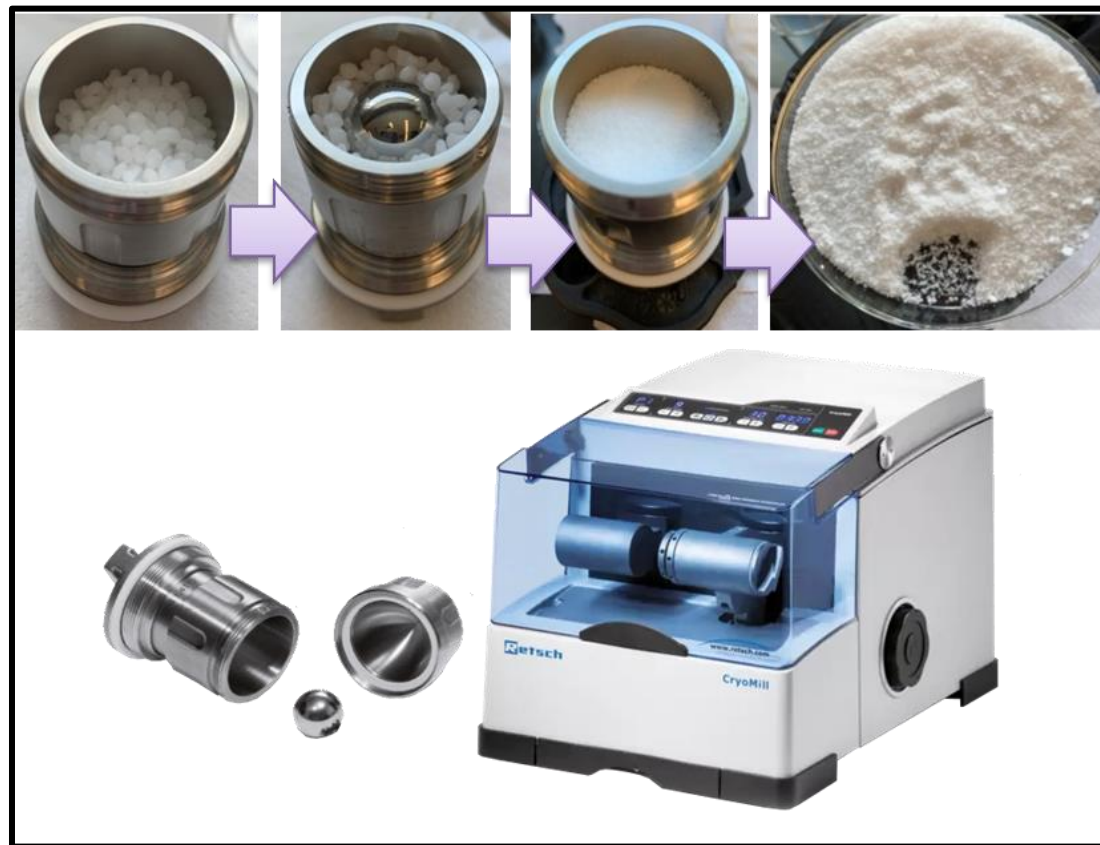
S_Figure 27. Cryomill used to process Virgin Plastics to Fine Powder showing milling jar with plastic pellets.
