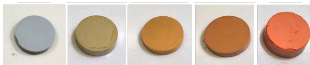
Figure 3-1. Photographs of \text{Ca}(\text{La}_{1-x}\text{Ce}_x)_2\text{S}_4 ( 0 \leq x \leq 1 ) samples show the color variation of x = 0.0, 0.25, 0.50, 0.75 and 1.00 compositions.
