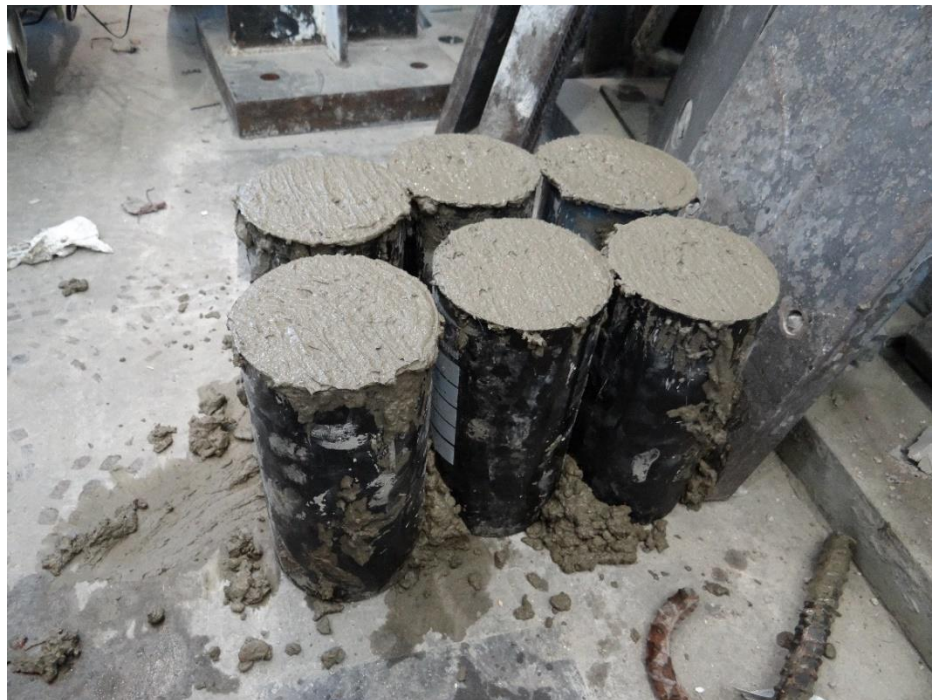
Figure 4-42 Concrete cylinders for test quality control
