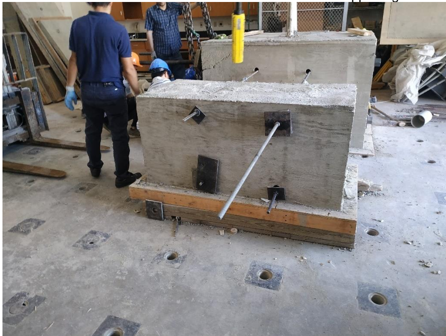
Figure 4-24 The North side view of the specimen while preparing to flip the specimen, four rods with 3/4- inch diameter were inserted to connect the supporting to loading blocks
