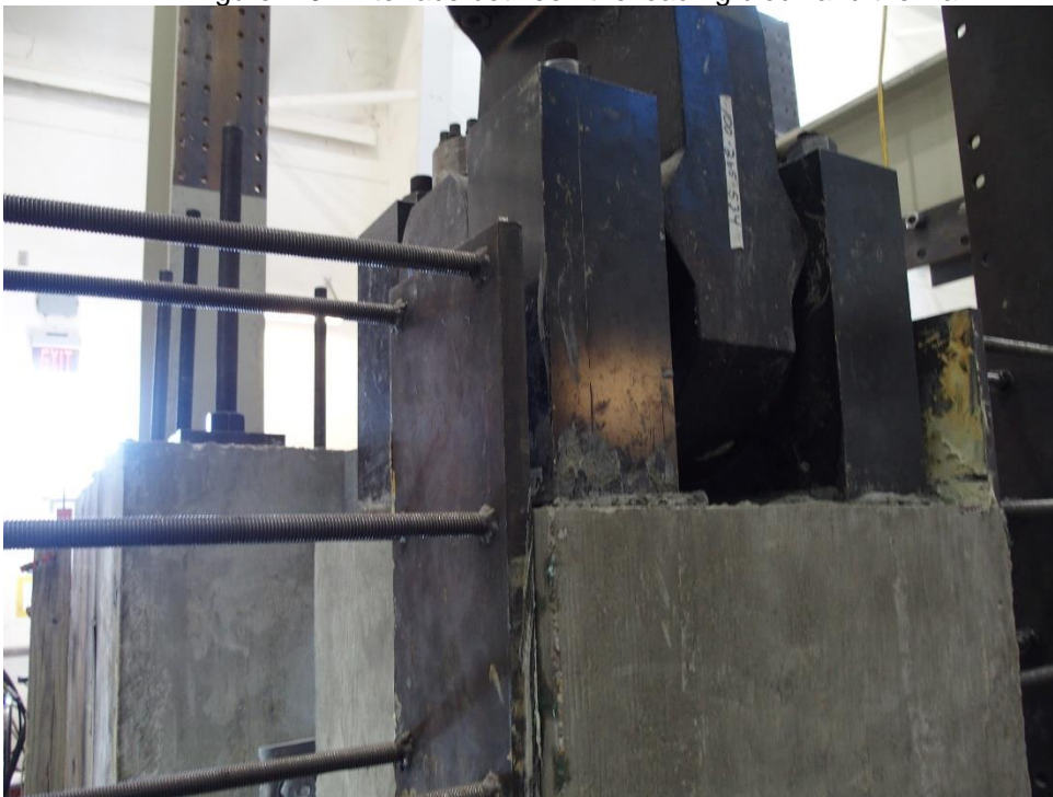
Figure 4-92 Connected actuator head to the loading block
