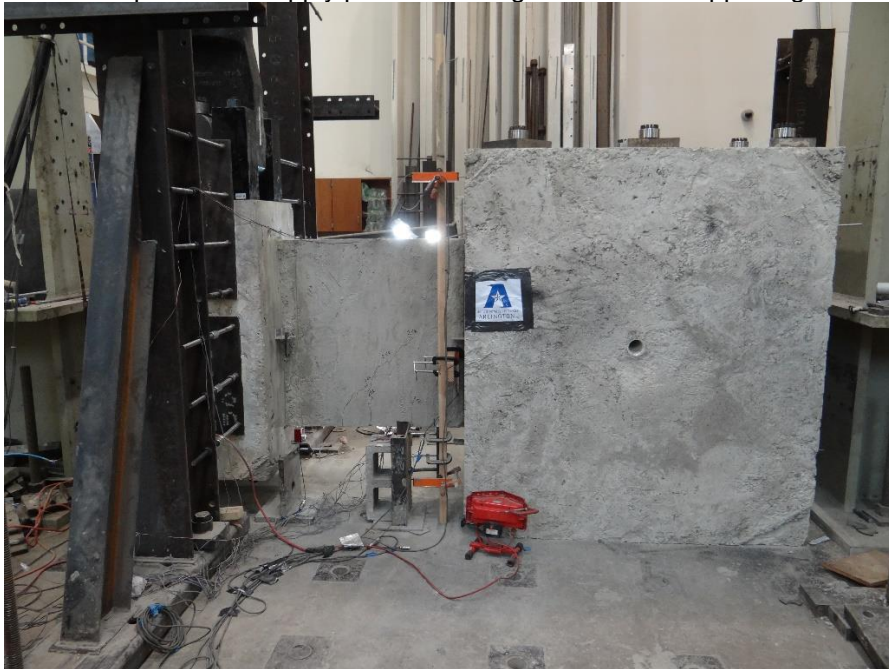
Figure 4-32 Two lateral bracing were used to prevent out-of-plane displacement for both sides of the loading block.
