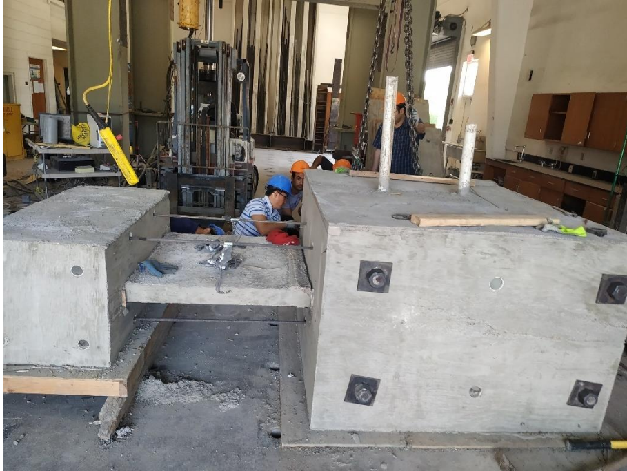
Figure 4-23 The West side view of the specimen while preparing to flip the specimen, four rods with 2-1/2 inch diameter were inserted in the supporting block
