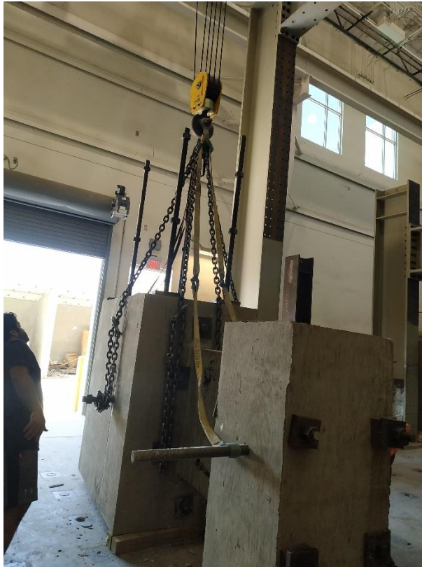
Figure 4-29 The specimen after flipping process was completed.
