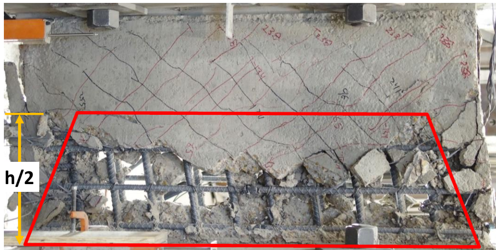
Figure 3-7 Failure mode of specimen SW-HA-0.5 at drift ratio 2%
