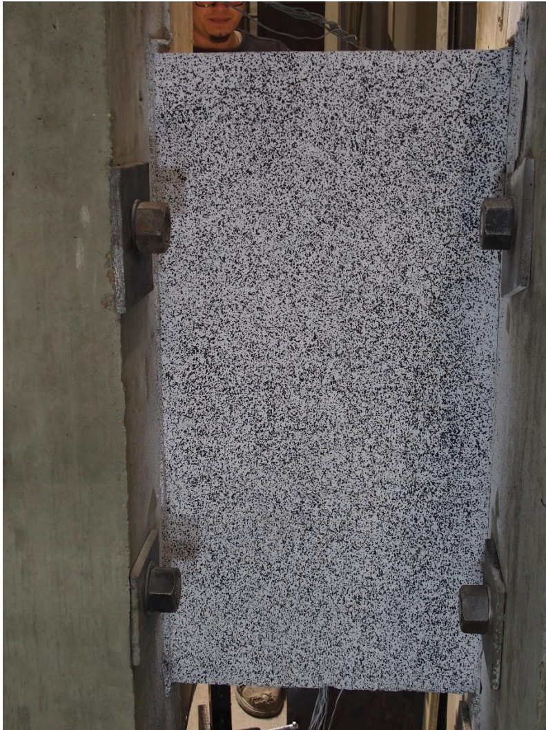
Figure 4-98 Wall face painted by White and Black dots.
