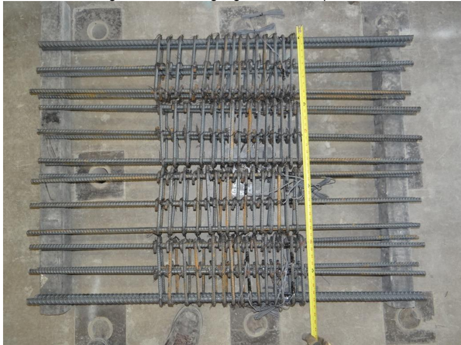
Figure 4-64 Steel cages to create a wall length of 40 inches.
