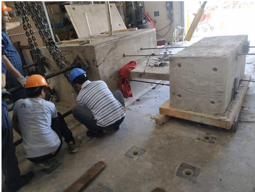
Figure 4-26 The East side view of the specimen while preparing to flip the specimen, four rods with \frac{3}{4} - inch diameter were inserted to connect the supporting to loading blocks plus four rods with 2-1/2 inch diameter were inserted to flip the supporting block by crane.
