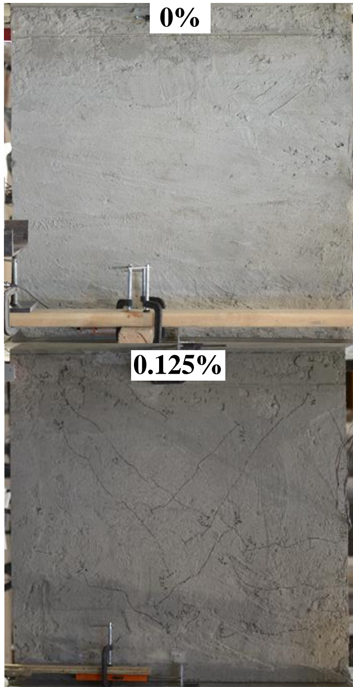
Figure 5-124 Test results of specimen SW-MA-1.0 at drift ratio 0.125%, 0.25%, 0.5%, 0.75%, 1%, 1.25%, and 1.5% (continued)
