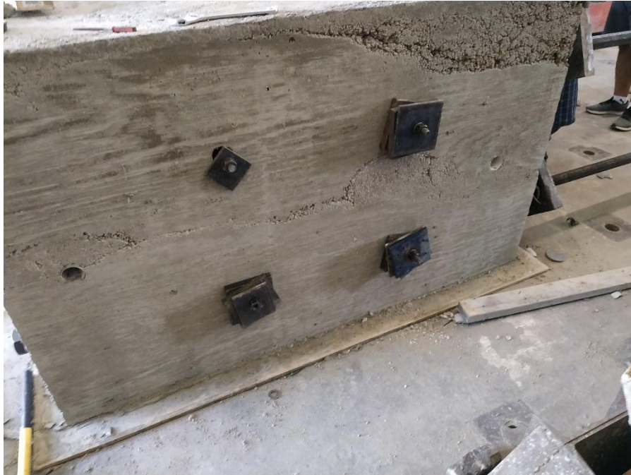
Figure 4-25 The South side view of the specimen while preparing to flip the specimen, four rods with \frac{3}{4} - inch diameter were inserted to connect the supporting to loading blocks
