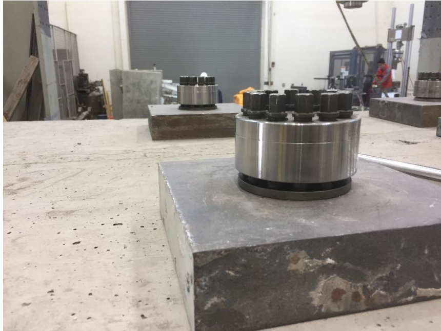
Figure 4-31 Super bolts to apply post-tensioning force on the supporting block rods.
