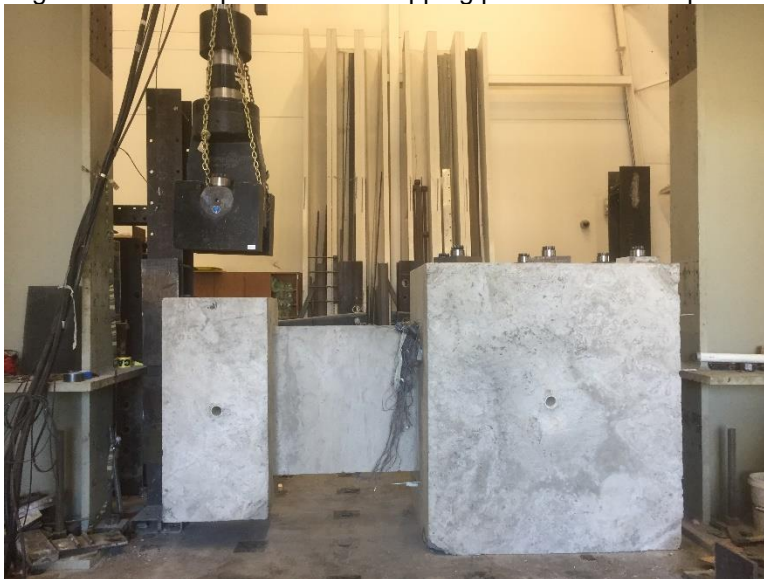
Figure 4-30 The supporting block was post-tensioned to the strong floor by six 2-1/2 inch diameter threaded rods, super bolts where used to apply 130 kips in each threaded rod.
