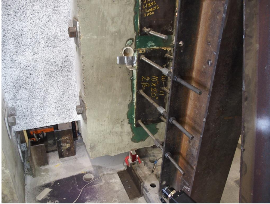
Figure 4-93 Lateral bracing frame
