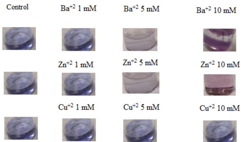
Figure 5.3.1: Ba +2 and Zn +2 ions were detected with liposomes as indicated by change in color. But for Cu +2 ions no change in color was observed
