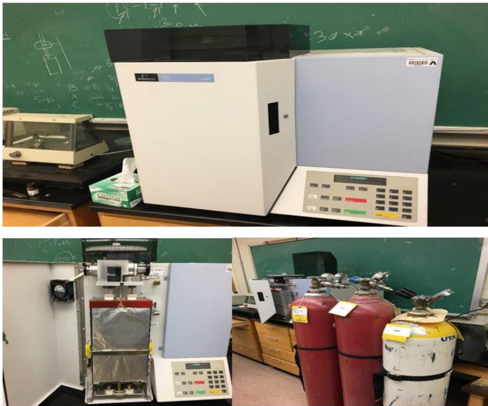
Figure 3-12 Components of elemental analyzer
