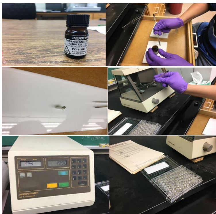
Figure 3-15 Sample preparation for elemental analysis
