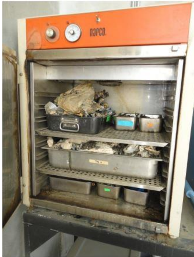
Figure 3-8 Moisture content determination by oven
