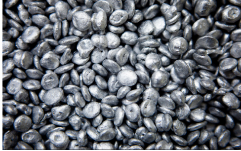
Figure 2-1: a) Aluminum ingot and b) pellet used to synthesize ACH.
