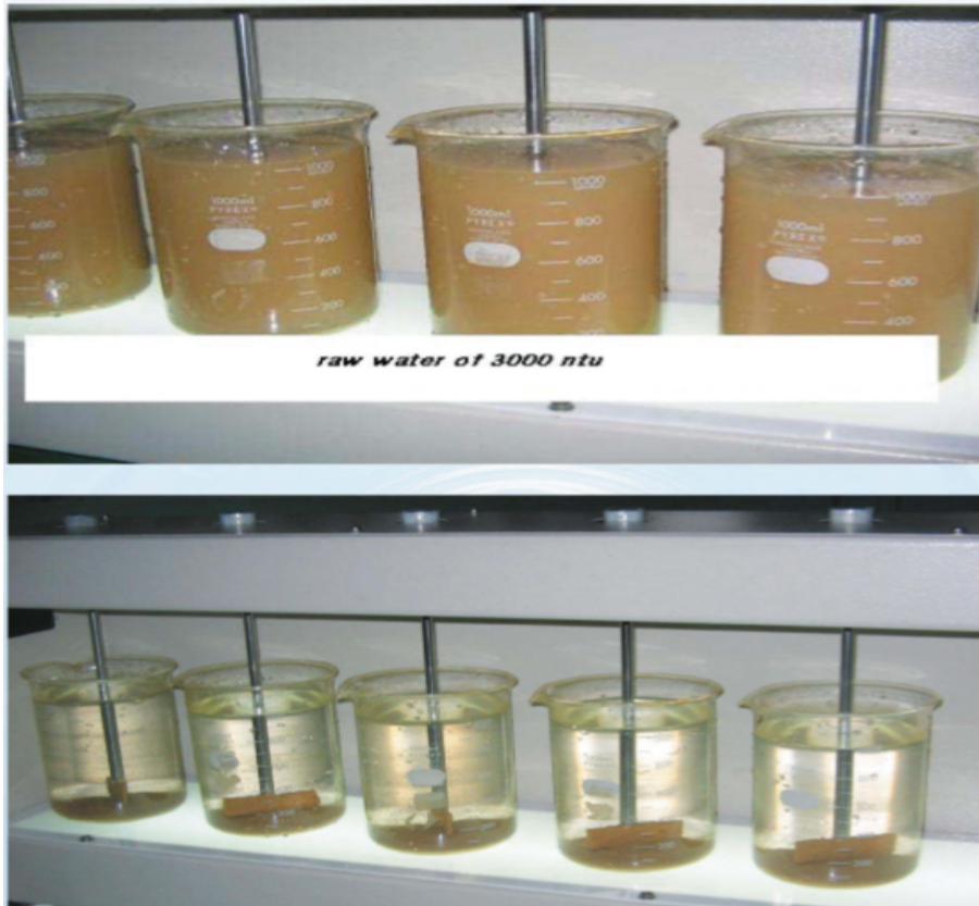
Figure 1-7: Effectiveness of aluminum chlorohydrate as a coagulant for water treatment. 29
