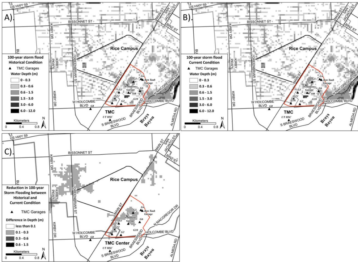
Figure 3.12: 100-year floodplain within the Harris Gully area under the Pre-(A)/Post-(B) improved stormwater condition and the flood inundation reduced depth(C).
