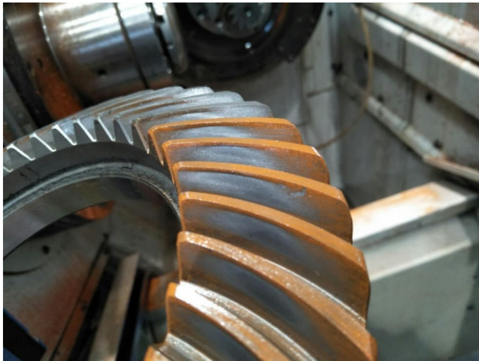
Figure 89 Contact pattern of design A test case on the coast condition
