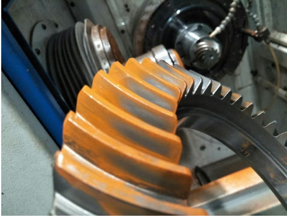
Figure 85 Contact pattern of design B test case on the drive condition
