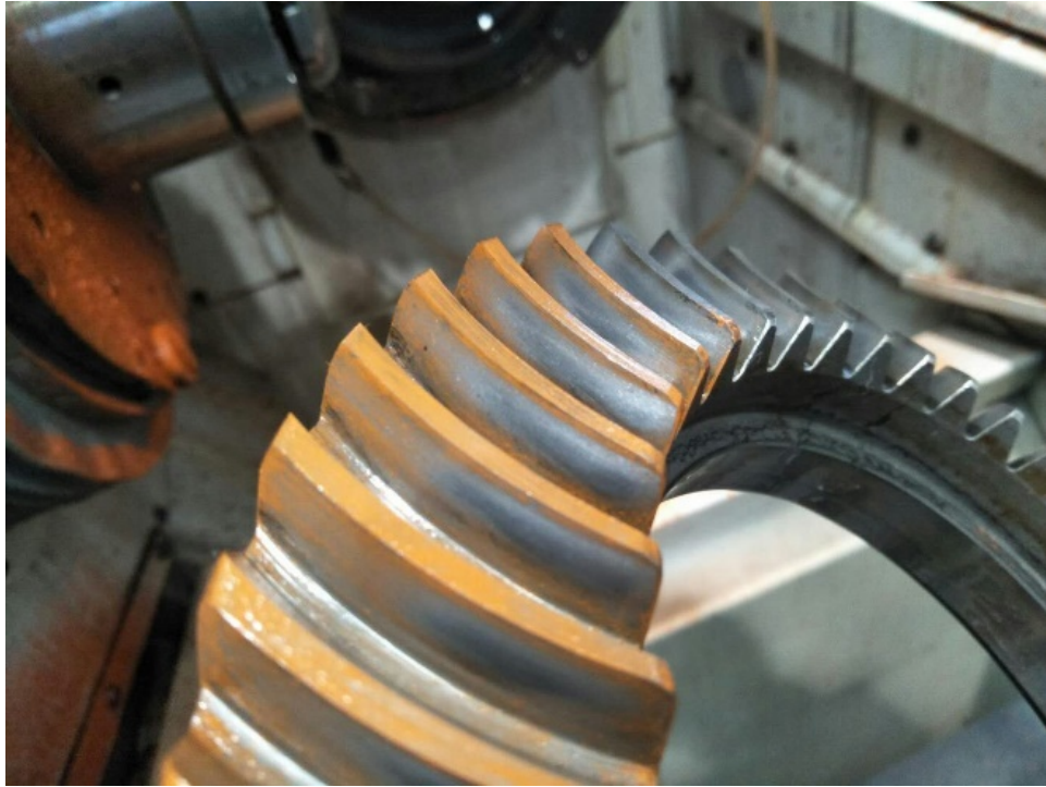
Figure 82 Contact pattern of design A test case on the drive condition
