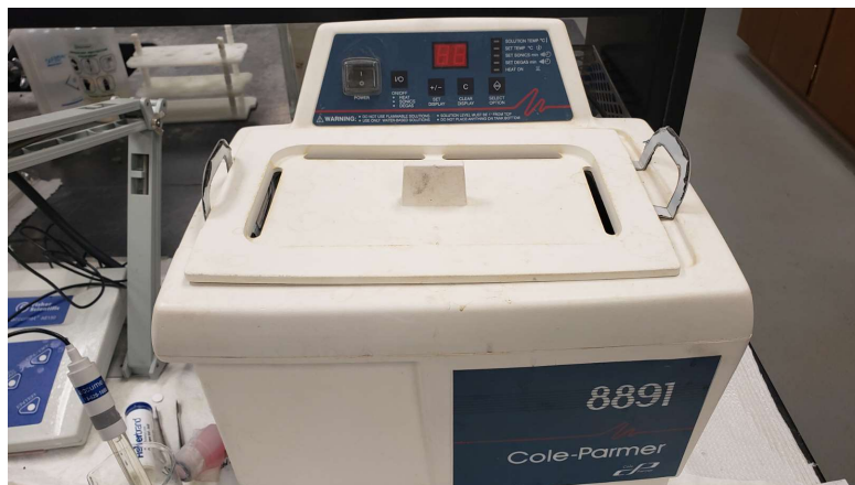
Figure 3-5: 8891 Cole Parmer sonicator used for desorption of target PFAS from solid phase present in reaction vials.
