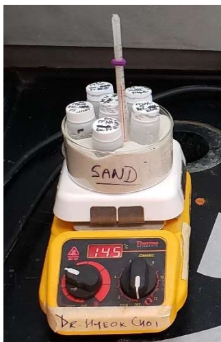
Figure 3-4: Sand bath utilized to conduct heated reactions.
