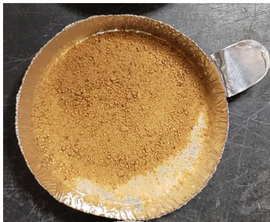
Figure 3-2: Aluminum dish loaded with soil and activated carbon for gravimetric characterization.
