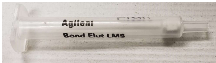
Figure 3-1: LMS cartridge utilized for sample cleanup. The cartridge is packed with a polymeric sorbent for separation of the target analytes.
