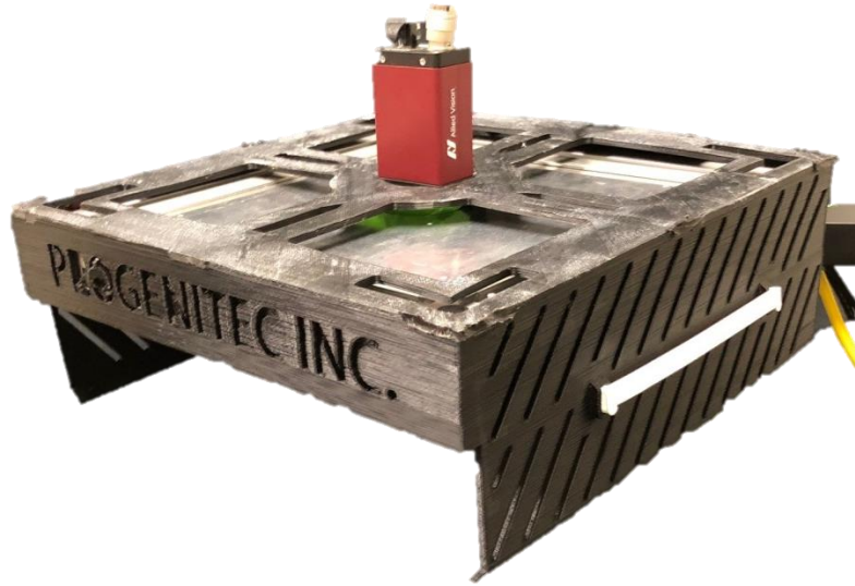
Figure 4.22. The R4 version of the 3D printed portable fluorescence imager design with CMOS camera and LED matrix mounted on an articulating arm.
