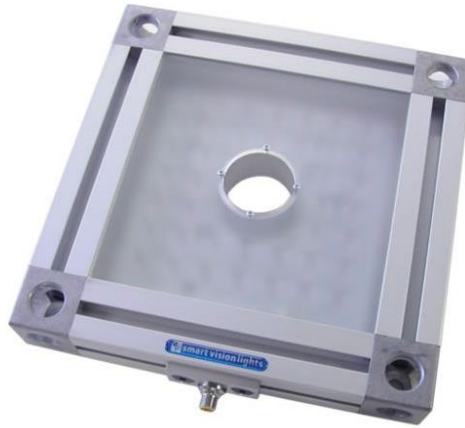
Figure 4.15. A 640 nm excitation wavelength version of the final LED matrix (© SmartVision).
