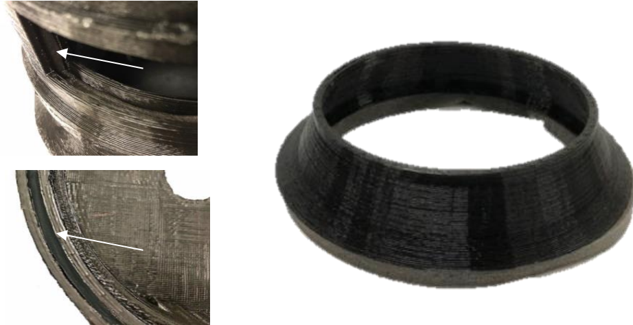
Figure 3.5 The locations of lightproofing gaskets that ensure light isolation during luminescence imaging is shown. These are integrated along the sliding white light shutter (upper left), where the top of the chamber connects to the exchangeable base (lower left), and along the bottom of the bases at the interface between the base and sample (right). These measures ensured complete light isolation during imaging.
