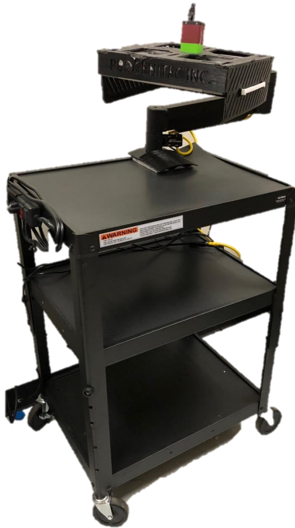
Figure 4.23. Example of the cart mounted R4 fluorescent (left) and luminescent (right) imaging devices. The articulating arm is fingertip-adjustable for ease of positioning.
