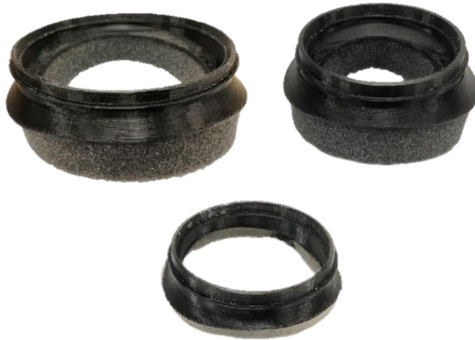
Figure 3.6. Detachable bases designed to account for anatomical curvature of a swine's dorsal area are shown.
