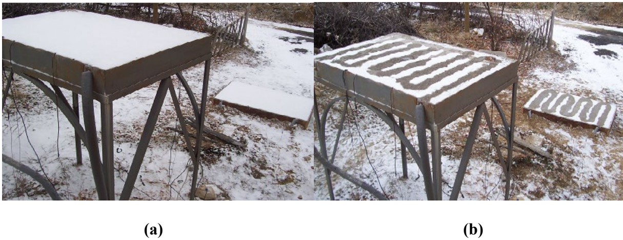
Figure 2-16. Initial and intermediate snow-melting process on slabs: (a) initial state ( t=0 ) for bridge and pavement slabs; (b) intermediate state ( t=30 min) for bridge and pavement slabs (Balbay and Esen 2010)
