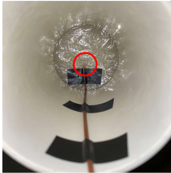
Figure 3.19 Thermocouple at the bottom of the compaction mold
