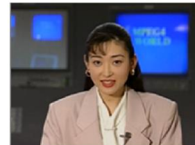
Output of EVC to HEVC transcoding (dec_HEVC.yuv) QP = 10, PSNR = 49.51 dB, SSIM = 0.9996
