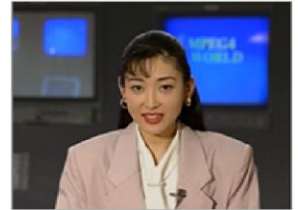
Output of HEVC to EVC transcoding (dec_EVC.yuv) QP = 10, PSNR = 50.00 dB, SSIM = 0.9996
