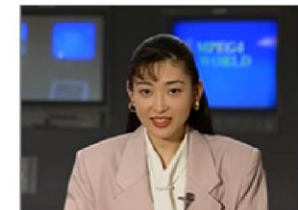
Output of EVC to VVC transcoding (dec_VVC.yuv) QP = 10, PSNR = 49.60 dB, SSIM = 0.9996
