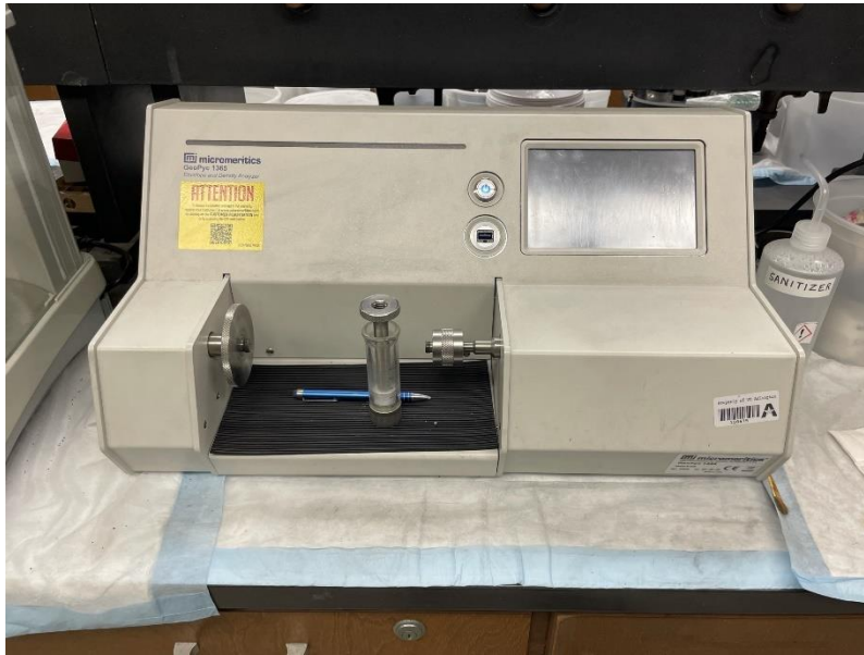
Figure 8: Micromeritics GeoPyc 1365 and a cylinder-shaped sample chamber
