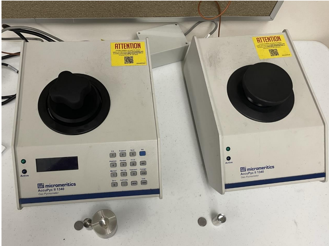
Figure 7: Micromeritics AccuPyc II 1340 with two different-sized sample chambers
