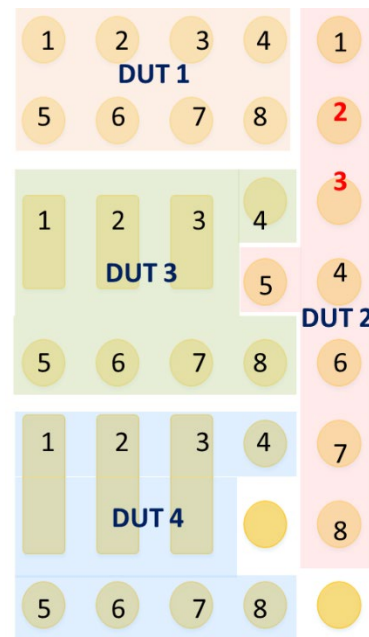
Figure 7-1. Schematics of DUT of second set of WCSP samples, showing different solder shapes.
