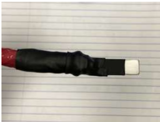
Figure 3.2: Example of insulated sample connected to electrode before processing
