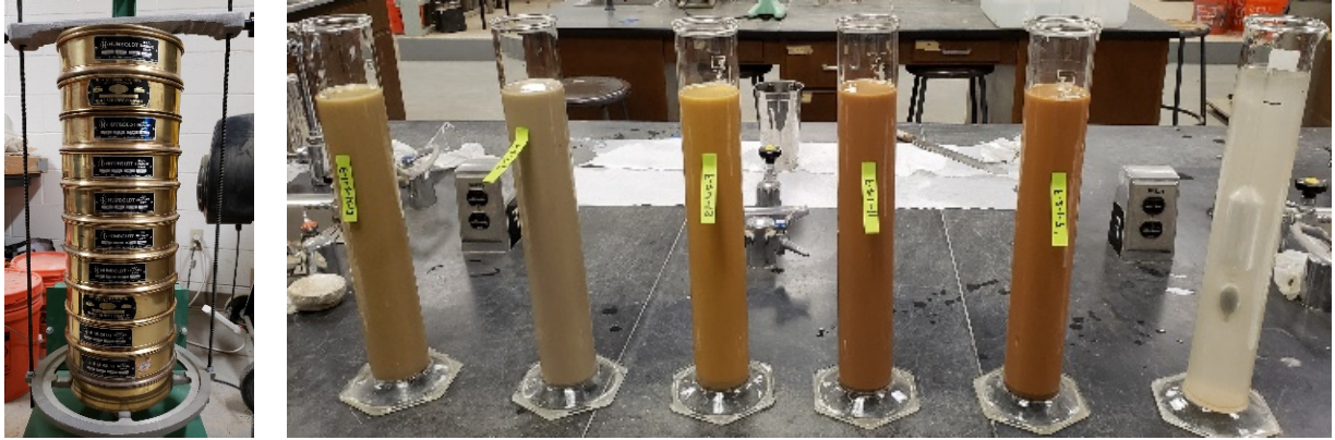
Figure 3-11 Grain size distribution (ASTM 422-63)
