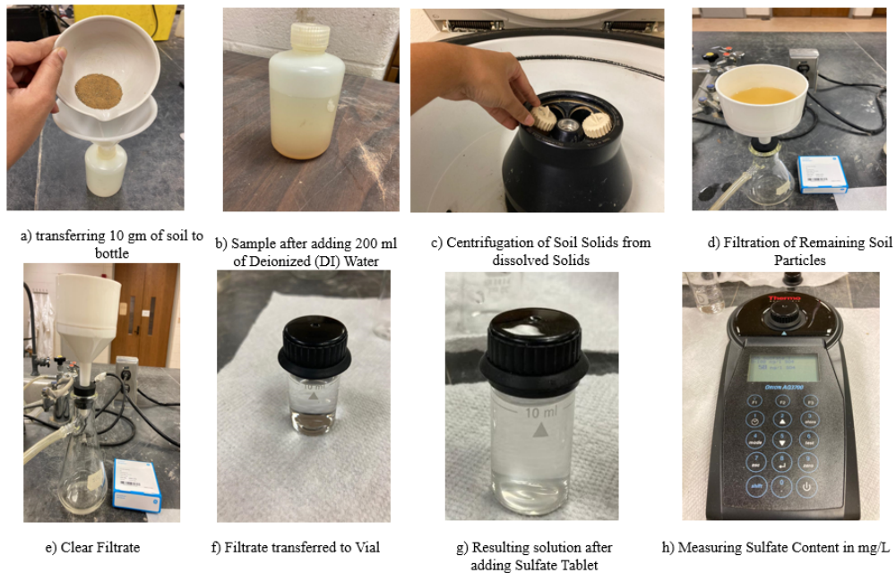
Figure 3-15 Determination of soluble sulfate of soil sample
