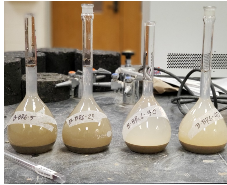
Figure 3-13 Specific gravity test (ASTM D854-14)
