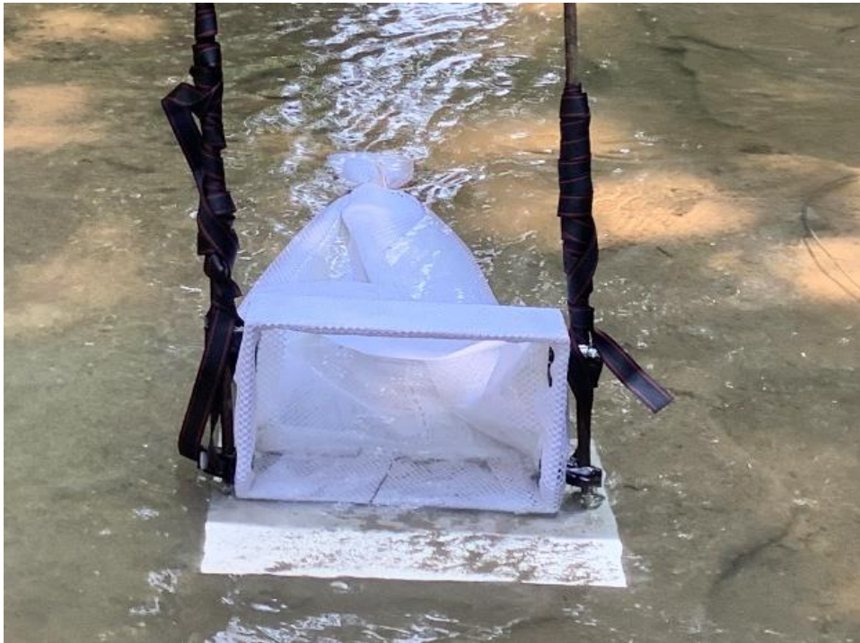
Figure 40 Bedload trap installed in Wilson Creek
