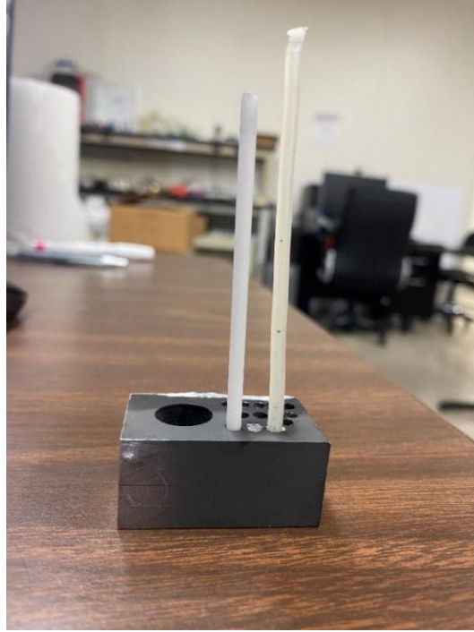
Figure 20. Design Fixture with Pebax filament on the left and Acetal on the right
