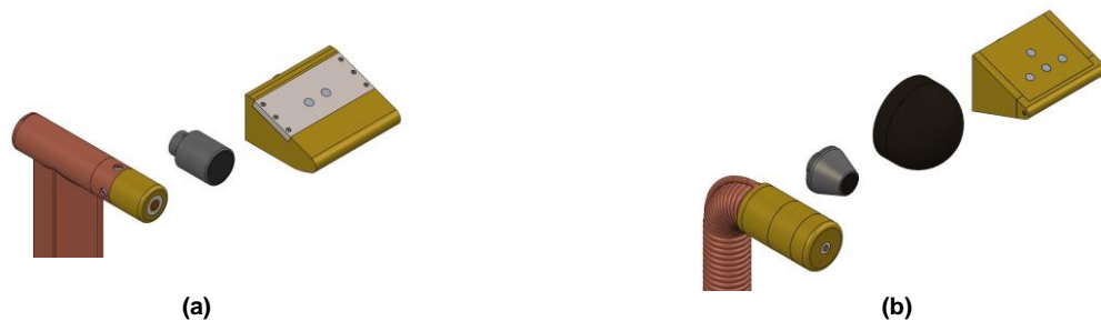
Figure 3-44: Slug-calorimeter, TPS material holder, and shear wedge for (a) Mach 4 conditions and (b) Mach 6 conditions.
