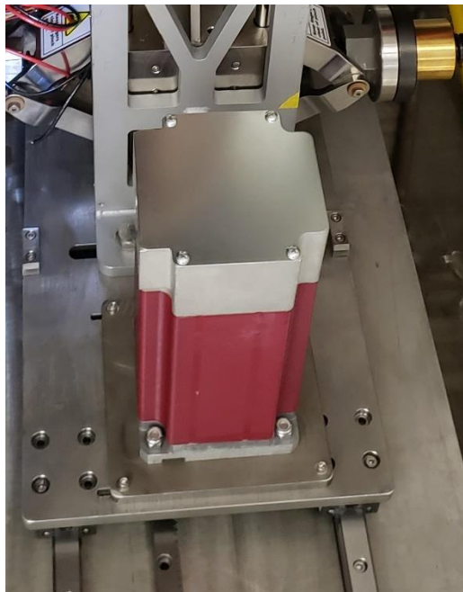
Figure 3-24: Carriage lateral motor during initial assembly.
