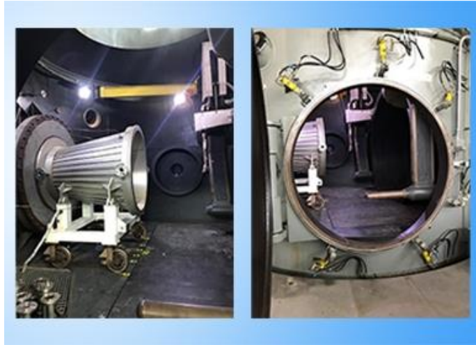
Figure 1-3: CIRA SCIROCCO Model Support System [10].
