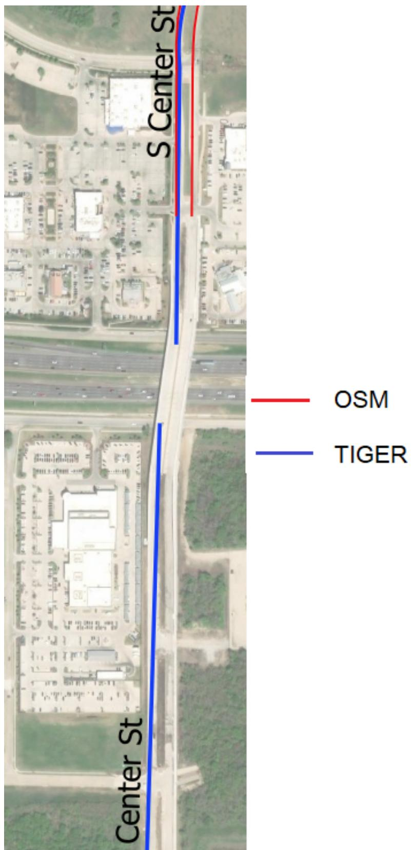
Figure 1.7: TIGER captures the extension of Center St while OSM does not
