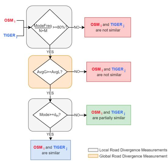
Figure 2.4: Flowchart of how to determine the similarity
