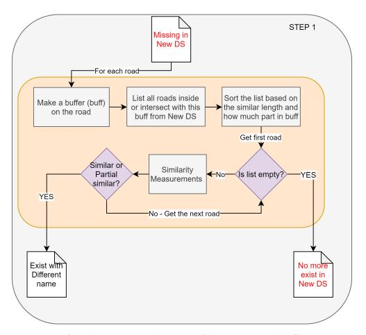
Figure 4.7: Check missing roads names if they exist with different names
