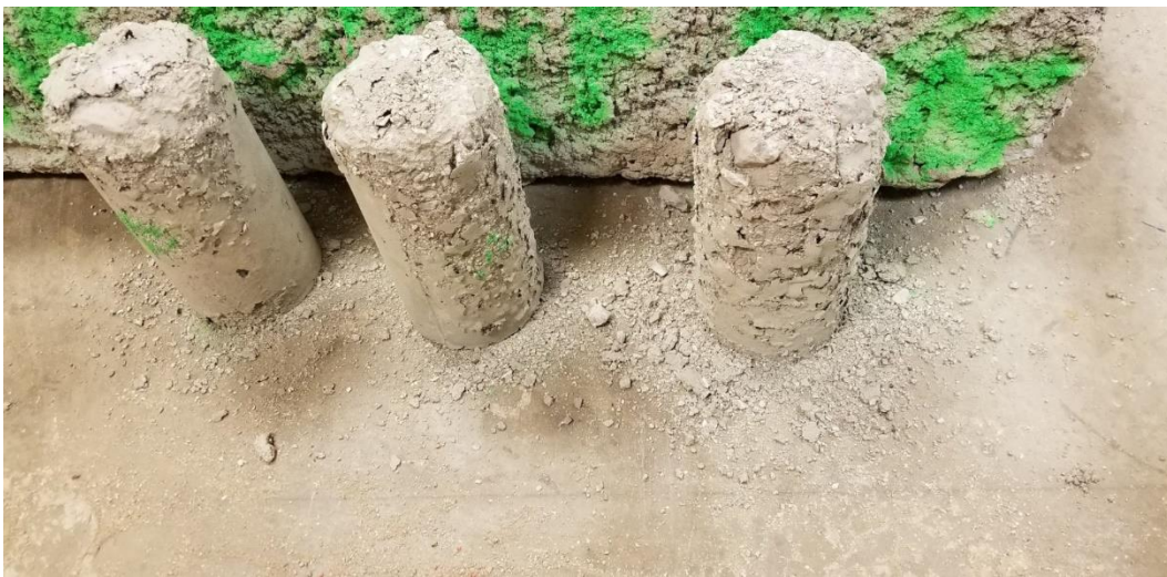
(b) Heat exposed damaged concrete cylindrical samples.
