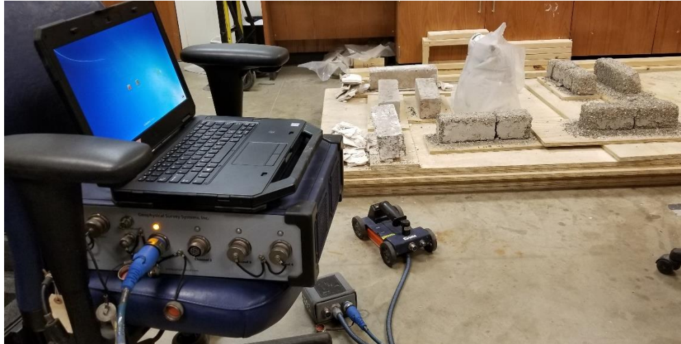
Figure 4- 35: Test setup for GPR scanning.
