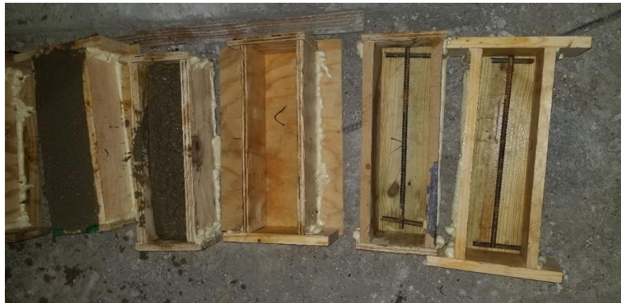
Figure 3- 1: Preparing preliminary study samples formwork and rebar placing.
