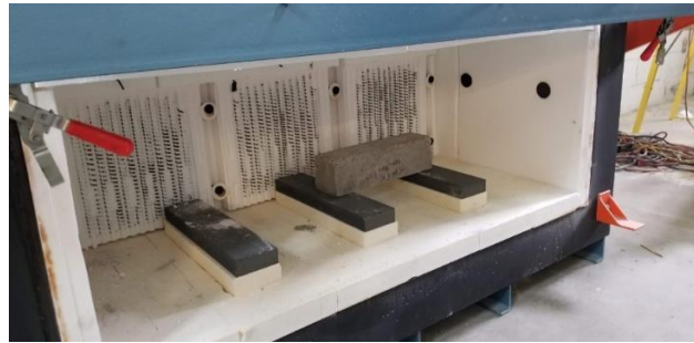
(b) Placing preliminary study samples in the furnace.
