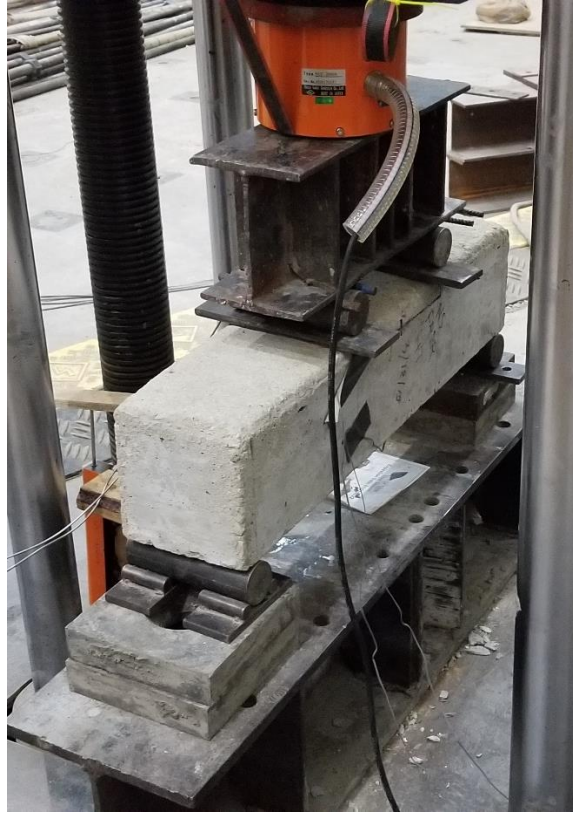
Figure 5- 3: Four point bending in laboratory.
