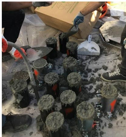
(b) Casting cylinder samples for the main study.
