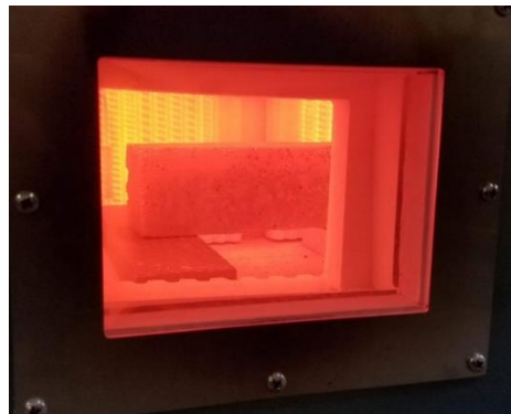
(c) Heat treating the samples.
