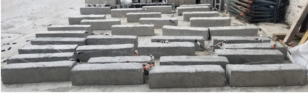
Figure 3- 7: Hardened beams after removing formworks.
