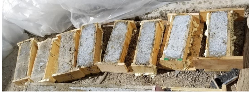
Figure 3- 2: Preliminary study samples after hardening and having curing compound applied.
