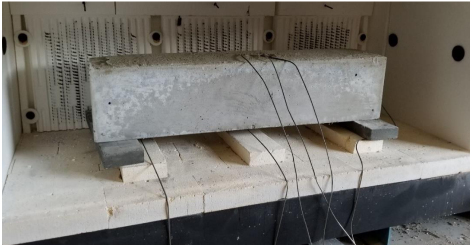
(b) Placing external thermocouples.
