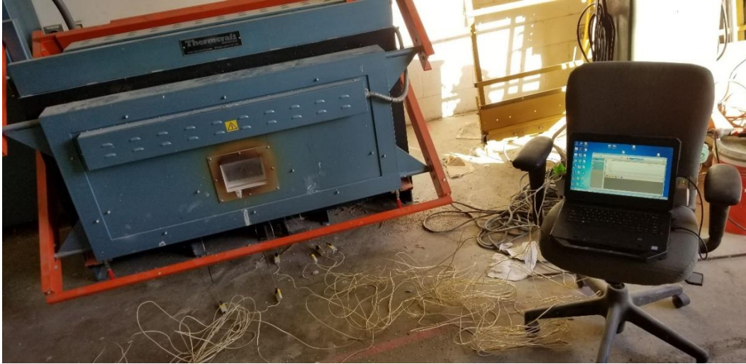
(c) Heat treatment setup with data logger and computer.
