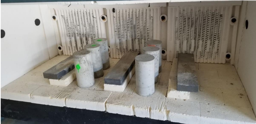
(a) Placing the cylinders in the furnace for heat treatment.
