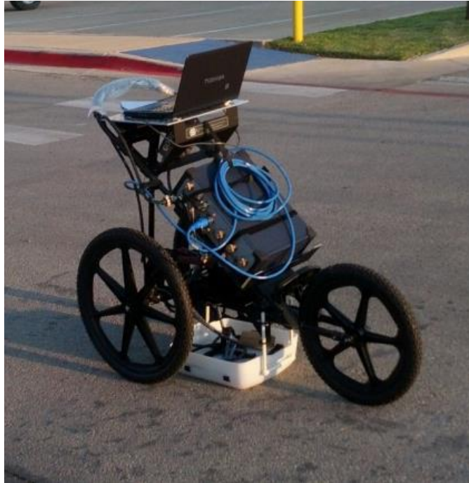
Figure 2- 4: Ground Penetrating Radar (GPR) on a Tri wheel cart setup.
