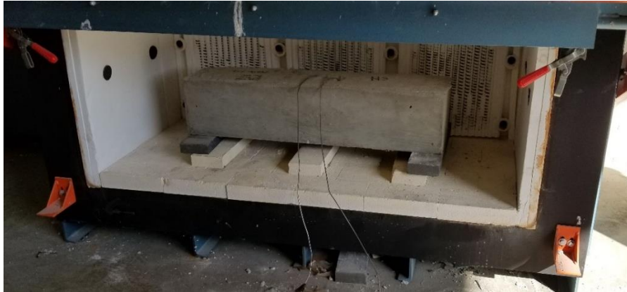
(a) Placing the main study beam samples in the furnace for heat treatment.
