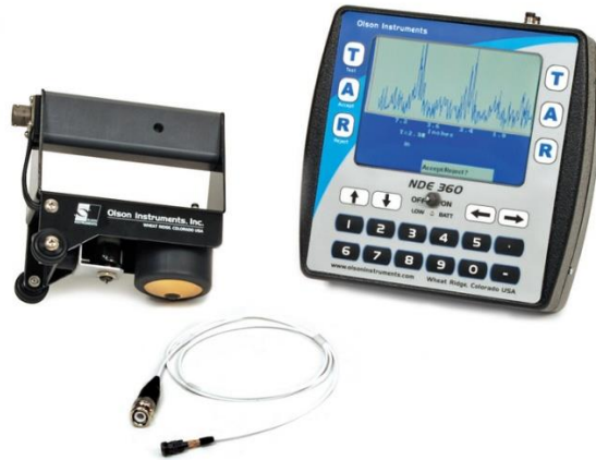
Figure 4- 24: Impact Echo (IE) device.
