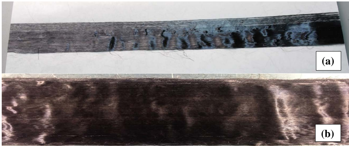
Figure 11. (a)Unidirectional prepreg tape (b) 1 st laminate: fiber misalignment in the first panel affecting the layup quality
