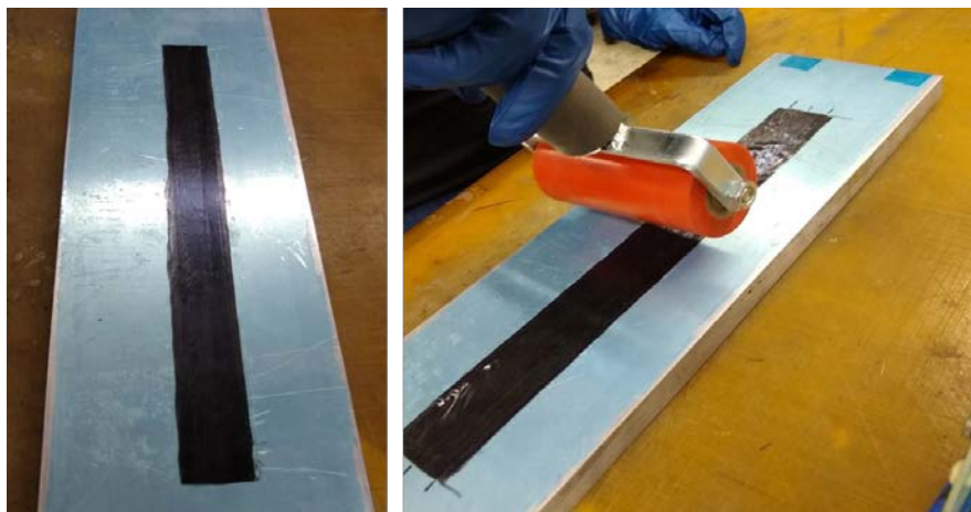
Figure 12. Layup process in the second unidirectional panel
