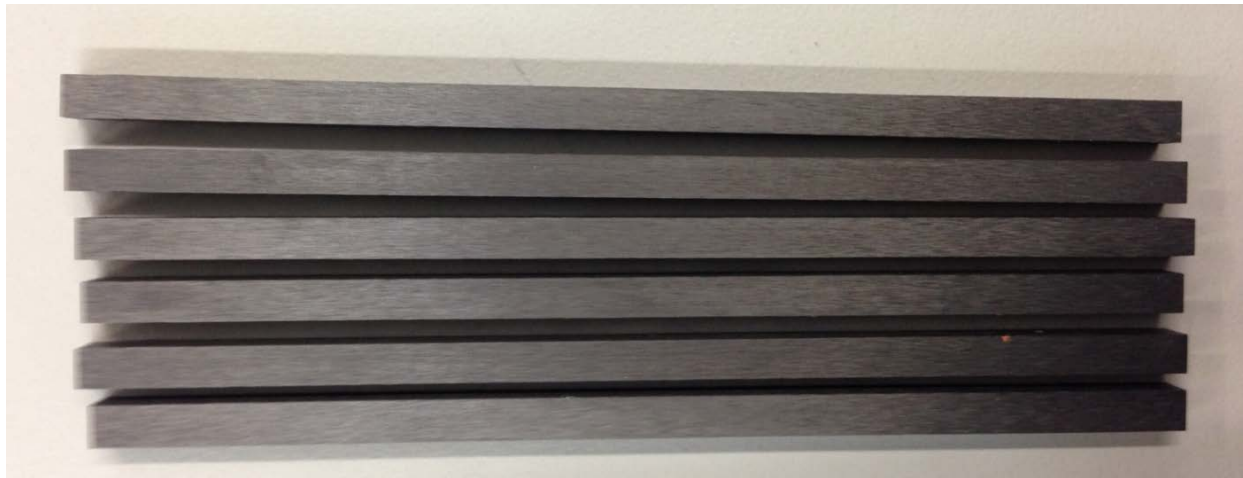
Figure 15. Unidirectional coupons for mechanical testing. The coupon dimensions are 3.88 x 0.16 x 0.16 in. (99 x 4 x 4 mm).
