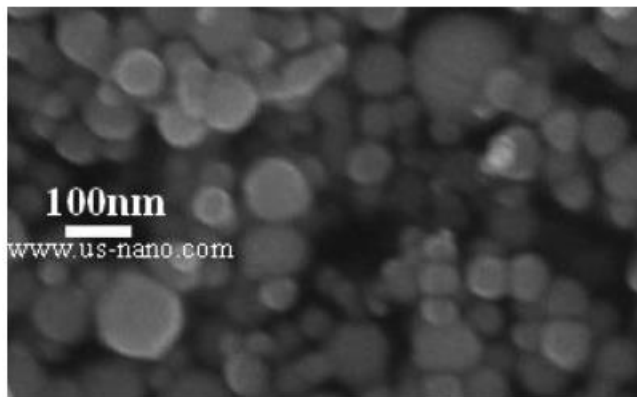
Figure 3-3 Copper Nanoparticles under SEM from US-nano research [36]
