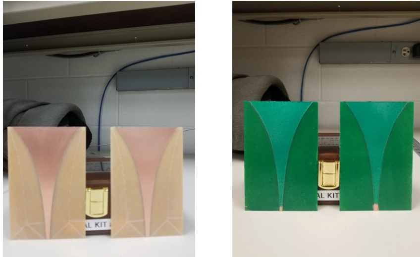
Figure 3.1: Sensor before and after surface coating
