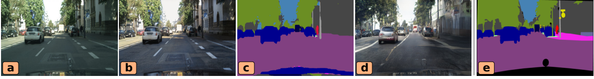
Figure 2.1: An example of our method on synthetic-to-real urban scene adaptation. Given a target-domain (or real) image (a), we first make target-to-source translation to obtain source-like (or synthetic) image (b), and then perform segmentation on these translated images. Our method improves the segmentation accuracy in the target domain by reconstructing both source and target images from their predicted labels (c). (d) illustrates the image reconstructed from (c), while (e) indicates the ground truth label.
