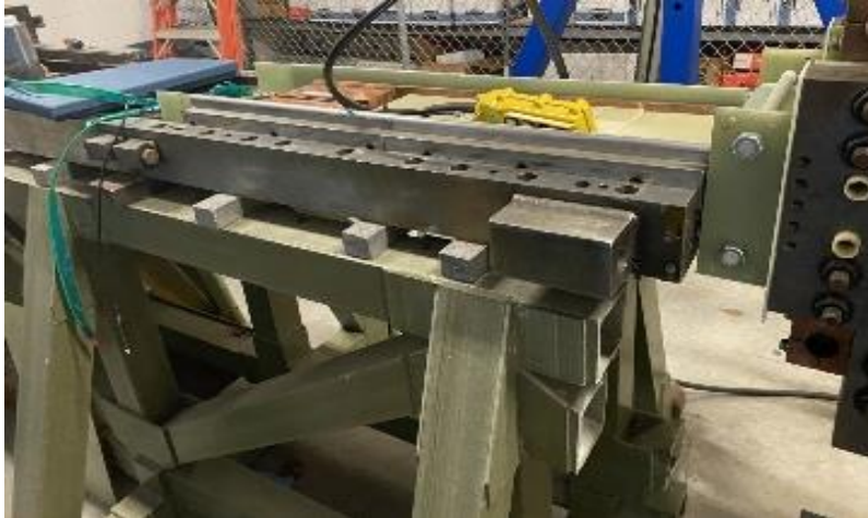
Figure 21 – Photograph of the 1 m section of the railgun testbench
