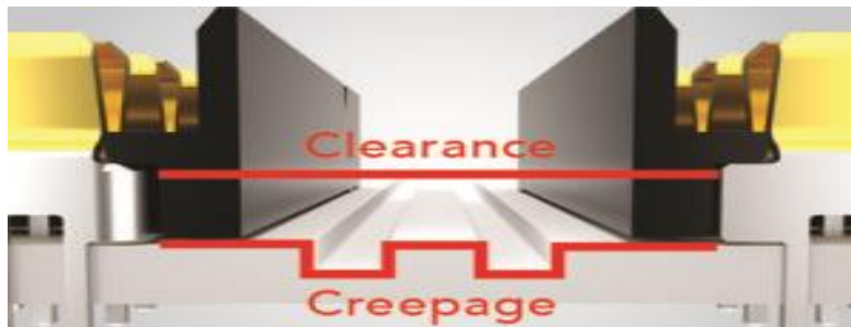
Figure 2 – Difference between creepage and clearance [11]
