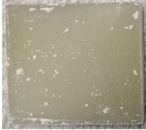
Figure 34 – Kaolin clay coated sample
