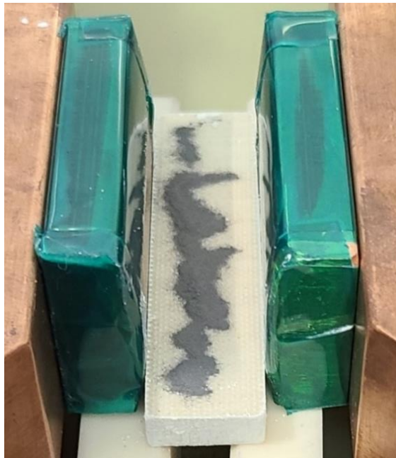
Figure 32 – Iron powder dusted sample prior to testing
