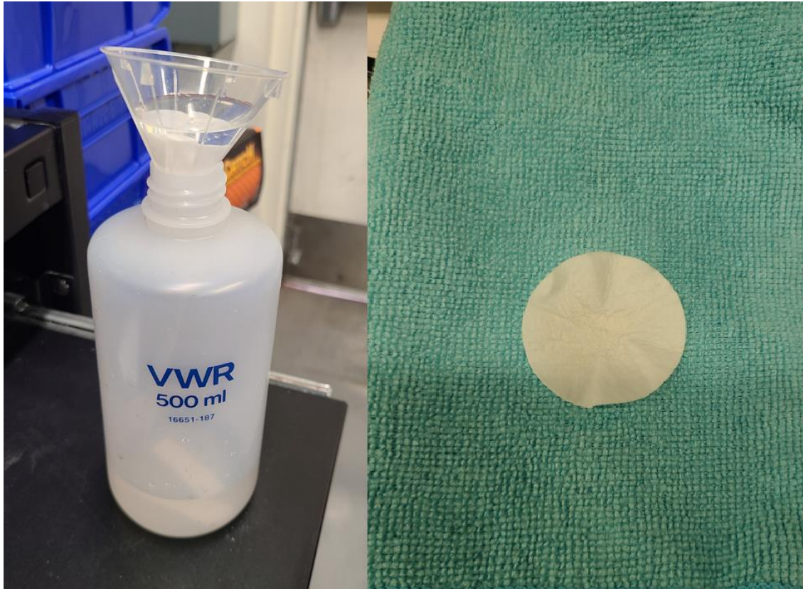
Figure 10 – Solution pouring through funnel and filter (left), filter drying with pollutants (right)
