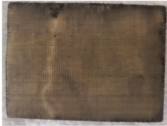
Figure 33 – Carbon dust coated sample after testing
