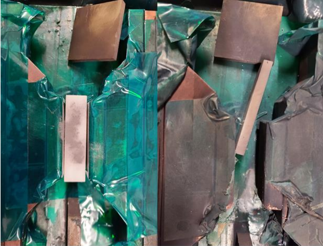
Figure 37 – Polluted Delrin® sample loaded into pulsed power testbench (left), after breakdown (right)
