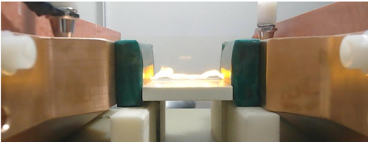
Figure 35 – Surface flashover of a polluted G9 sample
