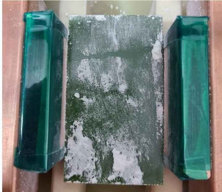
Figure 31 – Gypsum dusted sample after testing
