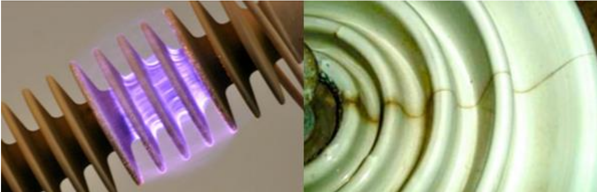
Figure 3 – Photograph of surface flashover occurring [12] (left) and its results [13] (right) on high voltage power line ceramic insulators
