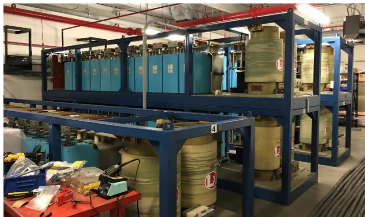
Figure 17 – Pulsed power supply capable of 1 MJ at 11 kV. 100 kJ at 11 kV operational
