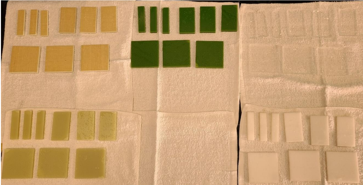
Figure 29 – NaCl polluted samples drying
