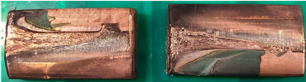
Figure 25 – Two-piece design electrodes after a breakdown
