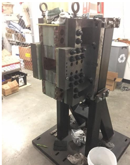
Figure 19 – Photograph of the high-current collection plates used to conduct current from the pulsed power supply into the flashover test setup
