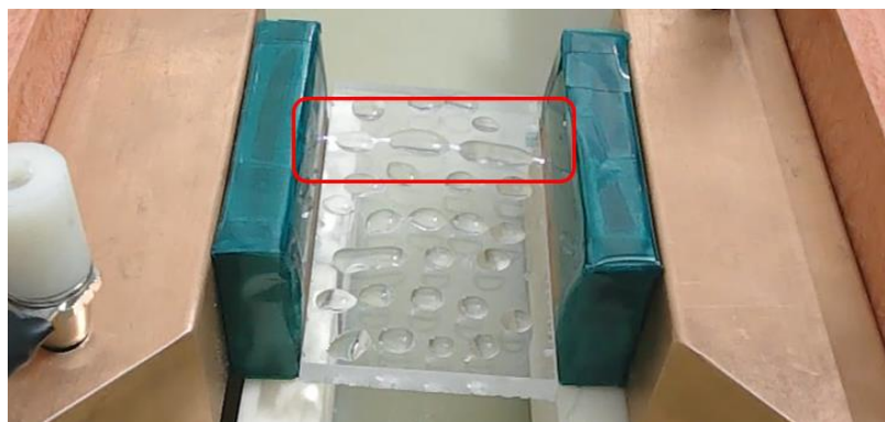
Figure 58 – Wet \text{NaCl} pollution breakdown on polycarbonate sample
