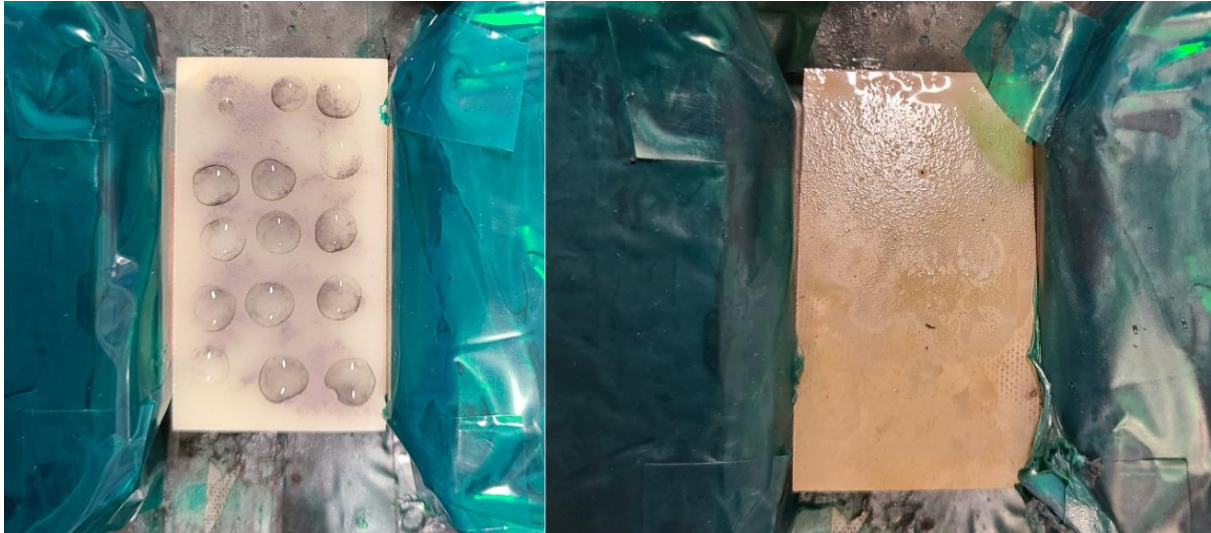
Figure 61 – G10 sample polluted with iron powder and water. Before breakdown (left) and after breakdown (right). The lower part of the sample, where the breakdown occurred, is completely dry – a dry band formed during breakdown. The top of the sample, away from the breakdown, is still wet.
