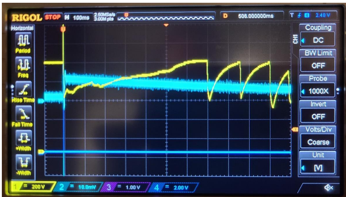
Figure 64 – G10 iron powder with water sample test. Oscilloscope readout from 3.5 kV trigger, 500 V below sample breakdown. Yellow curve displays voltage at 0.5X rate (2000X voltage probe with 1000X oscilloscope voltage probe setting), blue curve displays current at a reading of 0.1 V/mA. Probe reading displays voltage ringing without breakdown.
