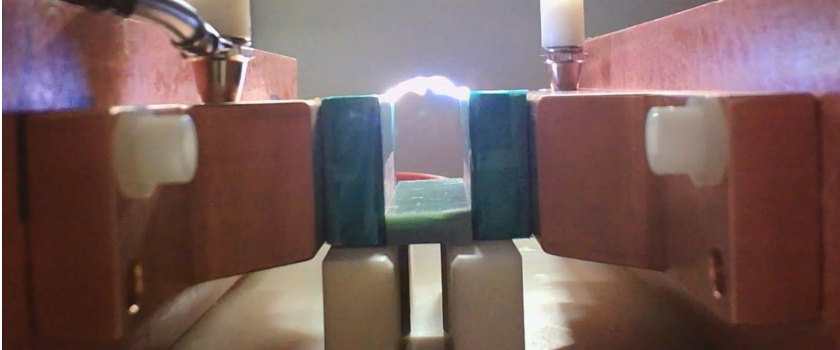
Figure 36 – Breakdown across the top of the electrodes
