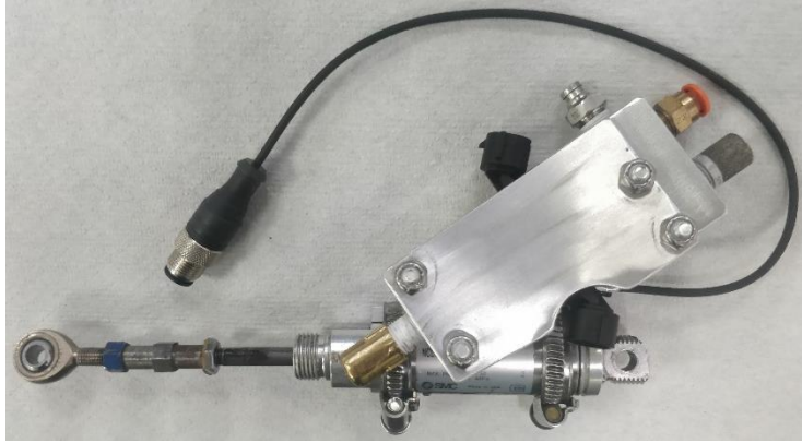
Fig. 2-23 Injector Block Mounted to Cylinder
