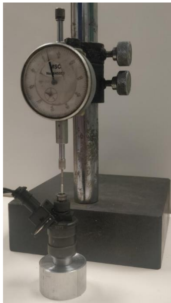
Fig. B-6 Measuring Injector Stroke
