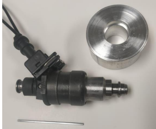
Fig. B-5 Aluminum Base, Fuel Injector, and Aluminum Rod used for Fixturing
