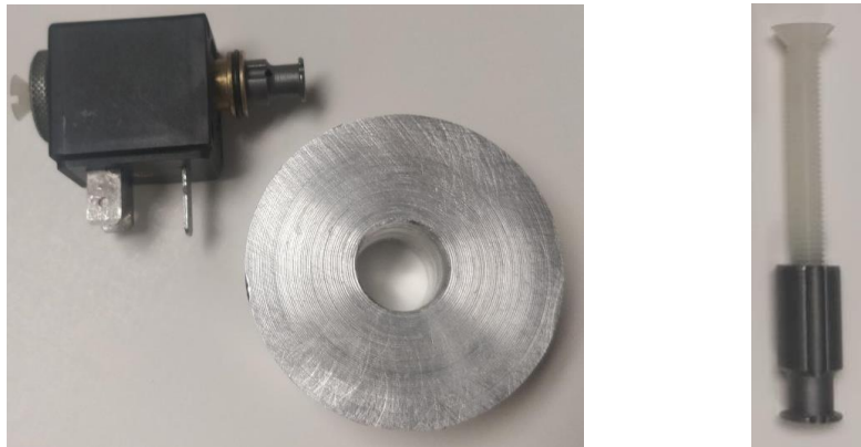
Fig. B-1 Assembled Solenoid and Base(left), Shuttle with added Nylon Screw(right)
