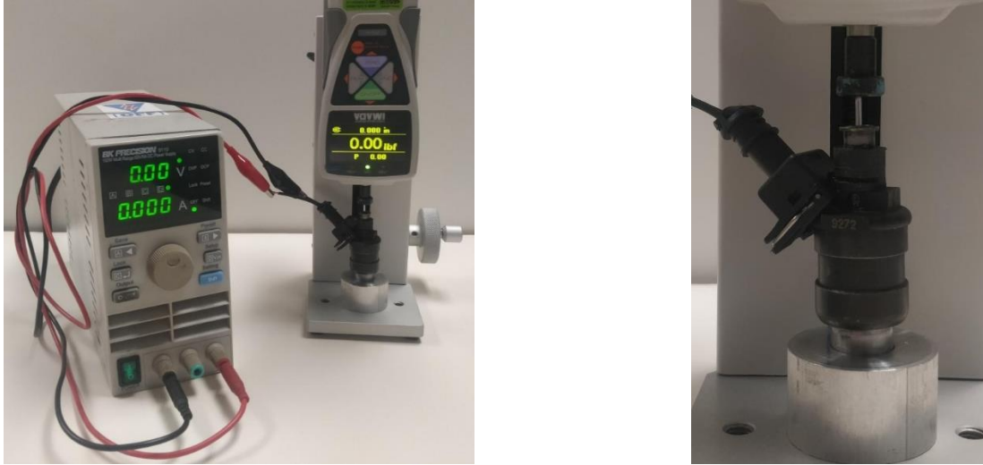
Fig. B-7 Injector Test Setup (left), Close-up view of Injector (right)
