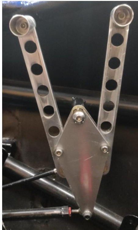
Fig. 1-1 UTA Manual Shifter Configuration, 1985-Present
