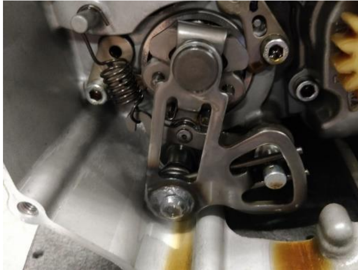
Fig. 1-2 Engine Shifter Ratcheting mechanism
