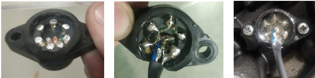
Fig. 3-4 Gear Position Sensor after machining (left), modified (center), installed (right)
